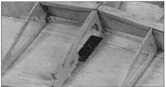
D 2. Cut out the aileron servo opening in the top center sheeting using the aileron servo cutout in rib R-6 as a guide. Make the opening slightly smaller than the servo cutout in the rib. The opening will be enlarged when the servo tray is installed.
