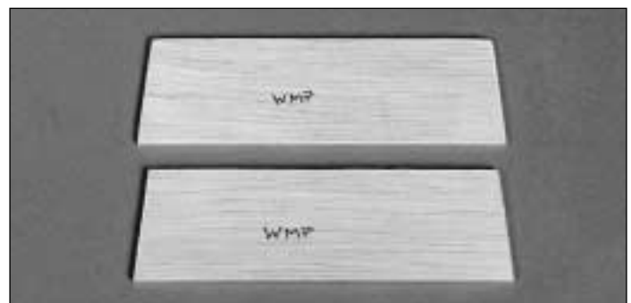
□ 36. Locate the two die-cut 1/8" [3mm] plywood wing mounting plates (WMP) . Glue them together to form one 1/4" [6mm] plate.
