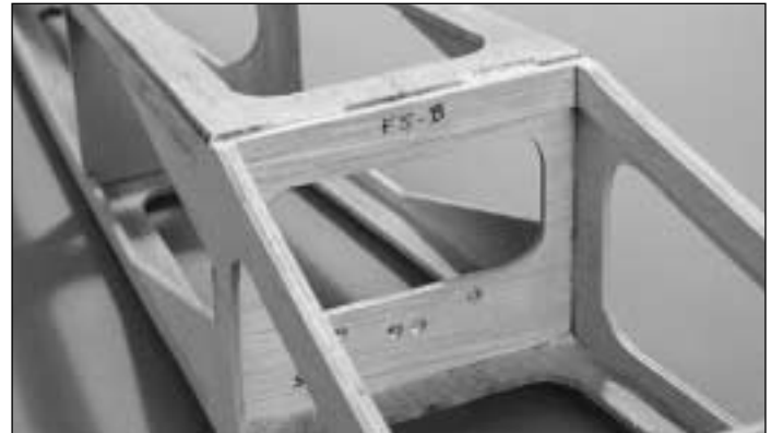
□ 35. Glue the 1/8" [3mm] die-cut plywood F5B to F5 as shown on the plan.
