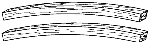
TWO WARPED SPARS INSTALLED THIS WAY WILL RESULT IN A WARPED WING
