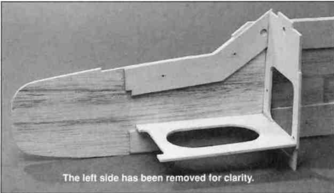
D 3. Insert the die-cut 1/8" ply tank floor between the fuse sides. The tab at the rear end should fit into the notch at the bottom of F-2 and the bottom of the tank floor should fit on top of the lower fuse doublers. Squeeze the fuse sides to the tank floor, then glue the tank floor in position with medium CA .
