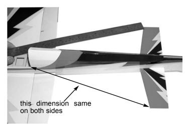
**4.** □ Use a ruler and measure from the tip of the stab to the front of the turtle deck and make sure the dimension is the same on both sides. When you have this the same the stab will be square with the fuselage.
