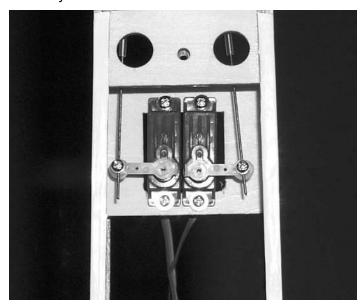
6. □ Put the pushrod in the hole in the pushrod connector and install arm on servo. Center the servos with the radio and make sure the rudder and elevator are centered. Tighten the screw firmly. Cut the excess pushrod off leaving about 1/2" past the connector. Don't forget to put the screw in the servo arm.
