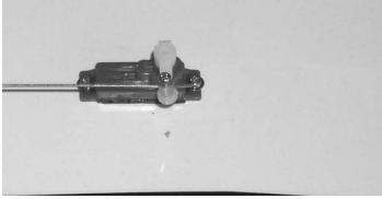
16. ☐ Insert the other end of the pushrod in the pushrod connector you installed on the servo arm. Install the arm on the servo. Center the servo with the radio and center the aileron. Tighten the screw on the servo connector. Install the screw to retain the servo arm on the servo. Cut the excess wire off the pushrod.
