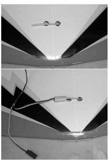
Tape one leg of the servo y-connector to the cable tie, string or soft wire.
