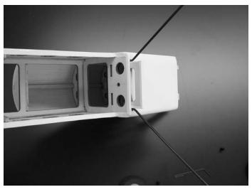
**4.**  $\square$  Take the landing gear cover plate and press into the slot on top of the gear. It is not necessary to glue in place.
