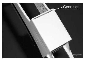
**2.**  $\square$  Remove the covering from the landing gear slot at the leading edge of the wing.
