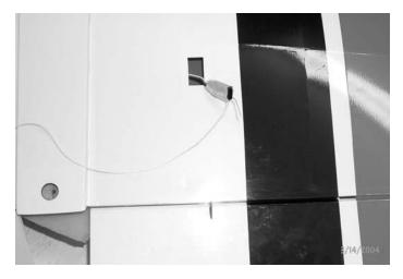
**10.**  $\square$  Carefully pull the aileron y-connector through to the servo opening.
