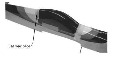
4. ☐ Place the canopy on hatch and tape in place till dry. Use wax paper at the rear to make sure you don't glue the canopy to the turtle deck.
