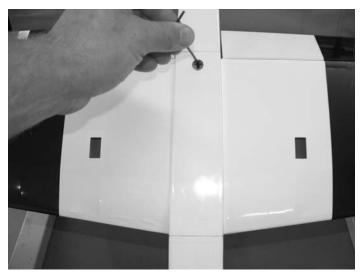
**5.** □ Bolt the wing in place using the 4-40 x 3/4" socket head screw.
