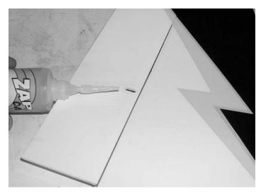
**6.**  $\Box$  Flip the wing over and glue the aileron horn from the top side of the wing using thin CA.
