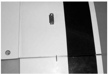
**13.**  $\square$  Screw the servo in place using the hardware supplied with the radio.
