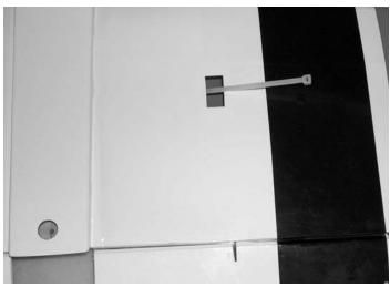
**8.**  $\square$  Locate the string, soft wire or a cable tie. Push it into the aileron servo cut out and fish it out the hole in the middle of the wing on the top side.
