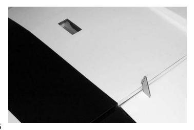
**4.** □ Install the control horn in the slot making sure that it is about 1/32" past the top surface of the aileron. Make sure the holes are aligned over the hinge line of the aileron.
