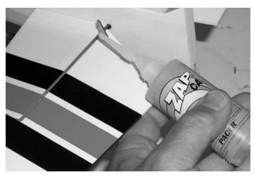
**13.**  $\square$  Glue in place using thin CA. Glue on top and bottom.
