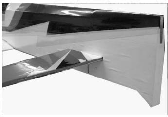
3. Slide the stab into the precut slot in the fuselage. Measure each side at the trailing edge to make sure it is centered.
