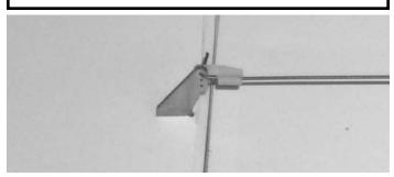
**15.** ☐ Make a 90 degree bend 1/4" long in the end of one of the 1/32 x 5-1/2" wires and install in the control horn. Use the nylon swing in keeper to retain the wire.
