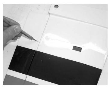
**3.** □ Use an X-acto knife or razor blade and remove the covering over the control horn opening. Do this on both sides of the aileron.
