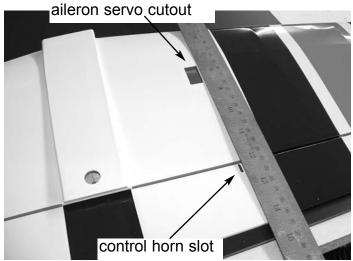
**2.**  $\square$  Locate the control horn slot by laying a straight edge along the outside edge on the servo opening. The slot is pre-cut in the aileron but is covered over with the film.
