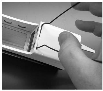
3.  $\Box$  Flex the landing gear legs together slightly and slide in the opening. Push all the way in.
