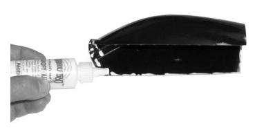
**3.** □ Apply a small bead of canopy glue around the edge of the canopy.
