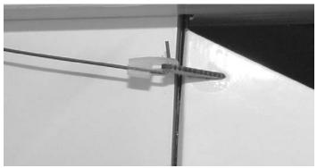
**4.** Use the nylon swing in keepers to retain the pushrod on the control horns.
