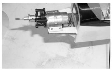
3. □ Place the top shell in place and secure using the four #2x1/2" screws.
