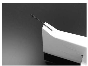
**6.** □ Drill a 1/32" hole in the tail skid mount 1/2" from the end. Insert the tail skid and cut a slot for the wire to fit into. Glue in place with medium CA.
