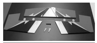
Caution: install the elevator joiner wire first.
