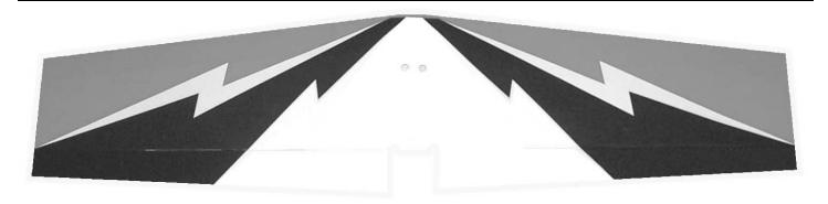
The wing for the Shock 3D comes pre-assembled with the ailerons already hinged. All that is required to finish the wing is to install the aileron servos, control horns and attach the pushrods.
