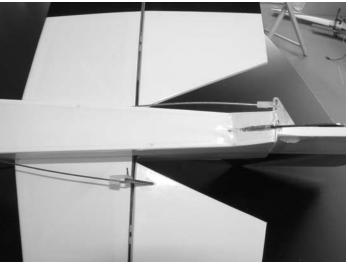
**5.** □ Install the two pushrod connectors on the control arms of the rudder and elevator servo as you did for the ailerons.
