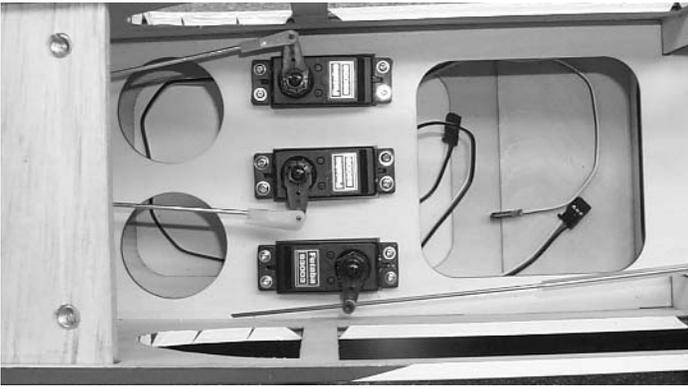
6.  Install the throttle servo into the servo tray.
