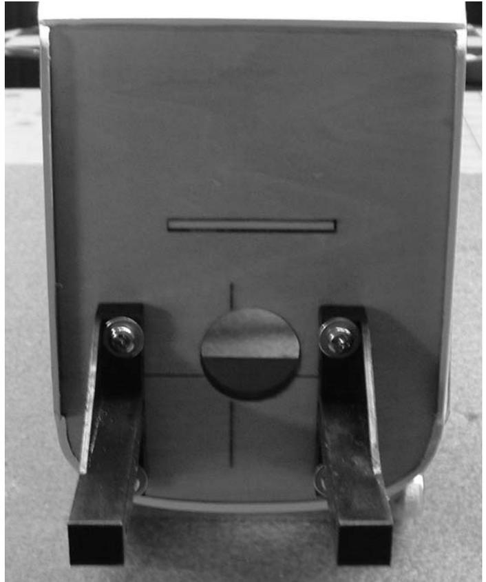
2.  Using thread lock, mount the motor mounts to the firewall using 8-32 x 3/4" screws with #8 washers.
