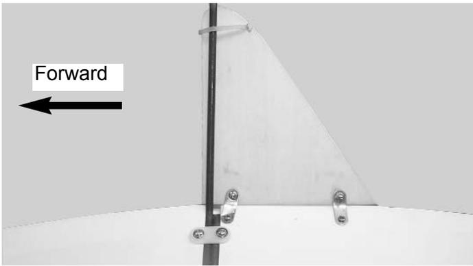
3.  Mount the fairing on the bottom of the plane as shown above.
