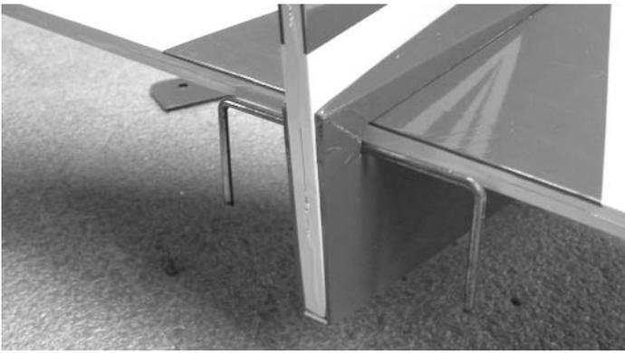
2.  Slide the fin mounting post into the rear of the fuselage.
