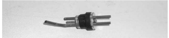
3.  Insert the brass tubes through two of the holes. They should be arranged so as the long one will be on the right side of the plane and the short one on the left side.
