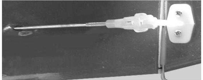
2.  Insert the rudder pushrod just like you did the elevator.
