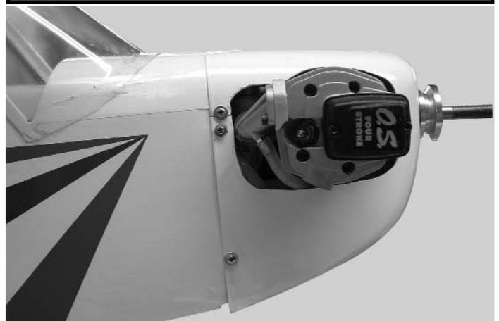
2.  Very carefully start removing the side of the cowl where the engine will protrude.
