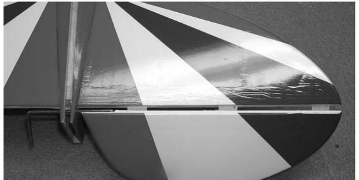
2.  Take three hinges and, as with the aileron hinge installation, insert the hinge into the elevator, using straight pins to ensure the hinge stays centered between the stabilizer and the elevator.
