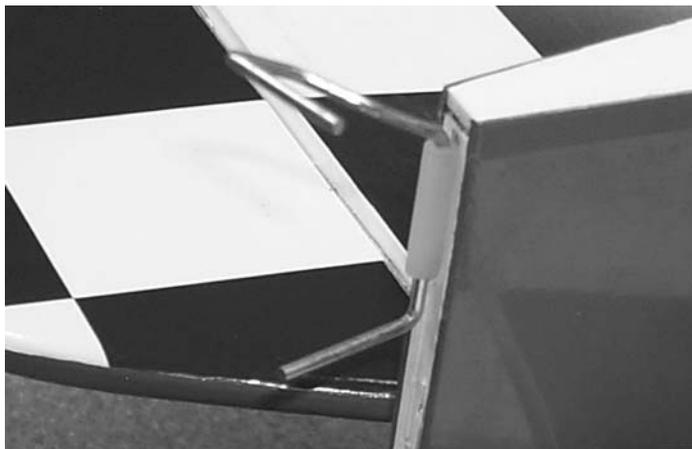
4.  Make a slot on the hinge line in the fin post for the nylon tail wheel hinge bracket.
