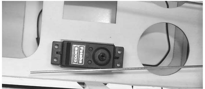
2.  Mount the elevator servo in as shown above.
