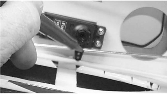
3.  Measure the length of the pushrod to the servo arm hole and make a 90 degree bend.
