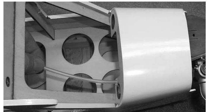
4.  Let the tubing exit into the fuselage towards the throttle servo mount.
