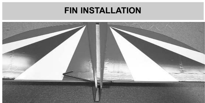
1.  Insert the elevator joiner in through the space behind the stabilizer slot.
