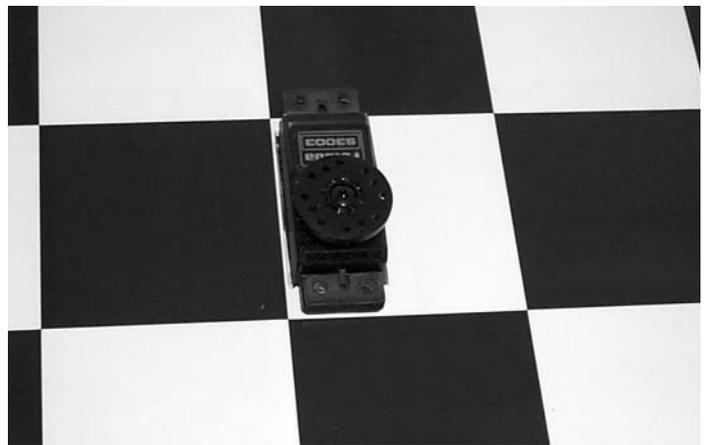
4.  Using the screws supplied with your radio, screw the servos to the mounting plates in the wings.
