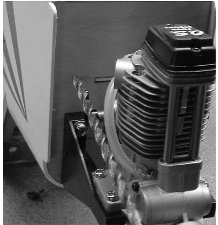
3.  Drill a 1/8" hole in the firewall in position with the throttle arm.
