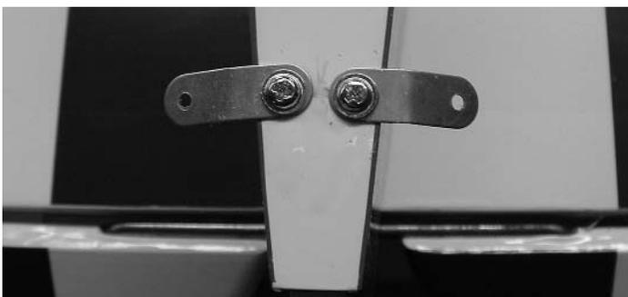
4.  Measure forward 1" from the rudder hinge line.
