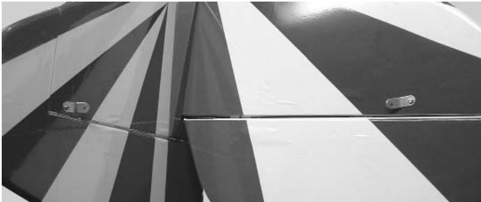
3.  The brackets go on each side of the fin and stab with one bolt holding two on. There is a predrilled hole at each location. Hold up to a light to help locate the hole under the covering.
