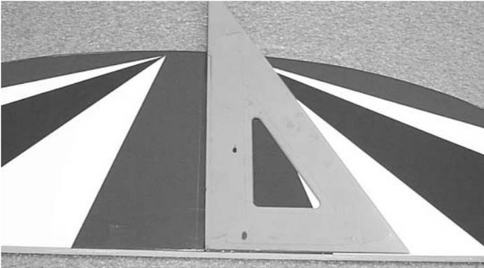
5.  From the center point on the stab, draw a vertical line up to the top of the stab.
