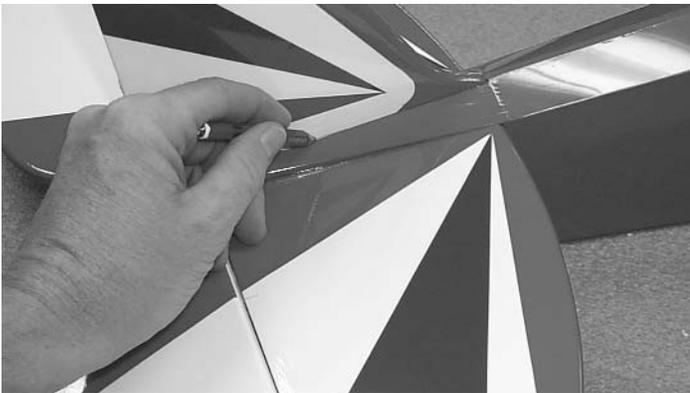
4.  When satisfied with the fit, mark the location of the fin on the fuse and stab by drawing a line on both sides of the fin, as shown.
