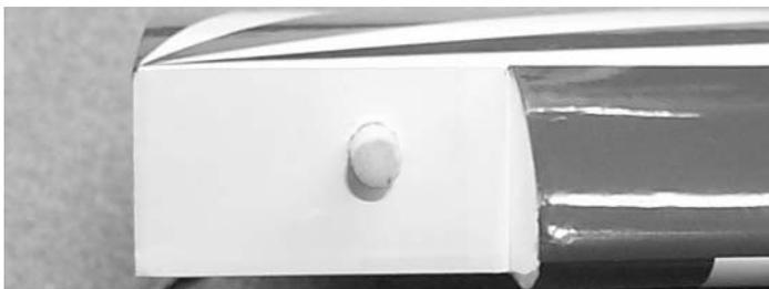
2.  Using epoxy, mount the 5/16 x 1-3/4" dowels into the holes in the notch of the leading edge of the wing. Make sure to leave about 1/2" of dowel sticking out of the front of the wing. You may wish to slightly taper the exposed dowel ends for ease of insertion into the fuse holes.
