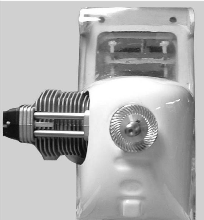
3.  Keep the hole in the front of the cowl centered on the engine.
