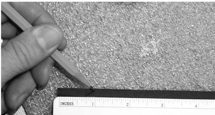
1.  Mark 1" up from the bottom of the rudder.
