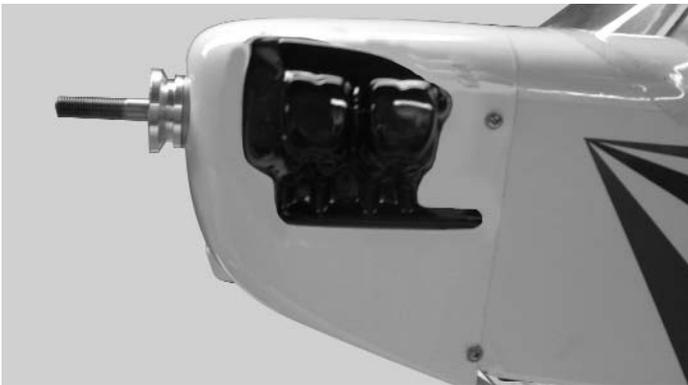
4.  Screw the cowl to the fuselage using #2 x 5/16 screws.
