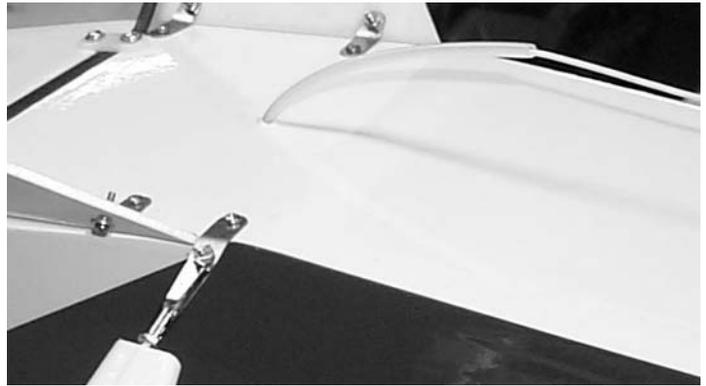
3.  Drill a hole in the bottom of the fuselage and extend the receiver out to the tail.
