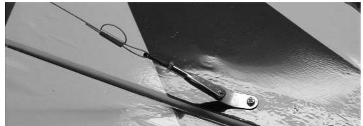
8.  Pass the cable through the brass tube, through the bracket on the stab and back through the brass tube.
