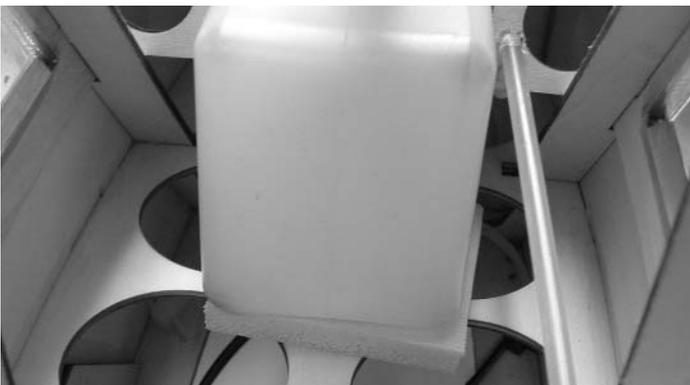
2.  You can insert some optional foam rubber under the fuel tank to help hold the tank in place.
