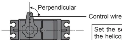
Set the servo horn length based on the helicopter manufacturer's instructions.
