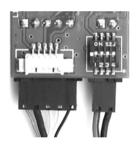
WARNING: DO NOT POWER TRANSMITTER WITHOUT ANTENNA ATTACHED. NO ANTENNA LOAD WILL DESTROY RF AMPLIFIER – NOT COVERED BY WARRANTY Small white connector on back of transmitter is for ImmersionRC Tiny Telemetry. See accessories.
