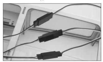
2. Plug the single lead from the wire harness into the gear channel of your receiver. An auxiliary channel can be used if the gear channel is occupied.
