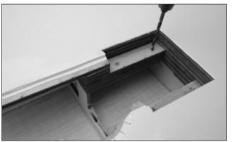
6. Install the retracts in the model using the screws provided with the kit or those of your own choice. A #4 x 1/2-inch wood screw works well. You will find the main units require the use of a 100-degree countersunk woodscrew while the nose unit requires a button head woodscrew.
