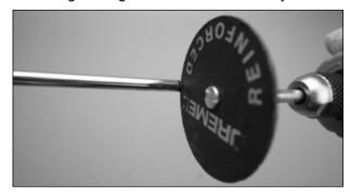
2. Make two flat spots on the end of the strut with a file and use a 2.5mm hex wrench to secure the axle to the strut. Apply threadlock to the threads of the retaining screws so they do not loosen from vibration.
