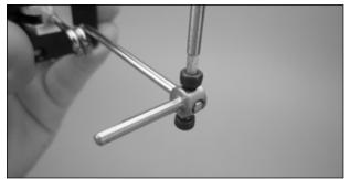
3. Install the wheels on the axles. Slide the brass wheel collar onto the axle and secure it using a 1.5mm hex wrench. Apply threadlock to the setscrew to prevent it loosening due to vibration.
