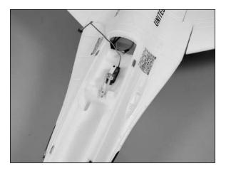
• 14. Locate the nose gear. Notice there is a slight bend to the gear wire. This bend will angle the gear forward in a scale-like manner when it has been installed.
