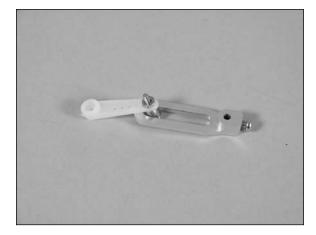
12. Remove the original servo arm from the servo Ο using a #00 Phillips screwdriver. After centering the steering servo, install the long 3D arm prepared in the previous steps on the servo as shown.
