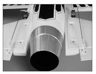
16. Repeat Steps 13 and 14 to install the 2<sup>7</sup>/<sub>8</sub>-inch (73mm) pushrod wire with clevis for the ailerons. The end at the servo will attach to the outermost hole in the aileron servo arm, and the clevis will attach to the outer hole on the control horn as shown. Make sure to install both the left and right aileron linkages at this time.
