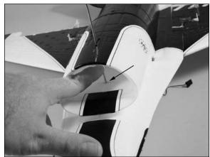
• 18. The nose gear will slide into the hole in the steering arm as its final destination. The screw at the steering arm will then be tightened so it is resting in the flat area as indicated back in Step 14. Use a #1 Phillips screwdriver to tighten the screw in the steering arm. Always remember to use threadlock on metal-to-metal fasteners to prevent them from vibrating loose.
