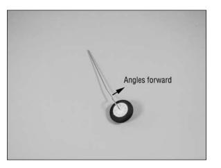
15. There are also two small flat areas on the nose gear that will face to the front of the aircraft. Please remember these flat areas for later in the nose gear installation.
