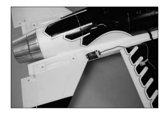
O 8. Connect a 9-inch (228mm) servo extension to the lead on the elevator servo. Tie a piece of string or dental floss around the connection to prevent the two from unplugging accidentally. Install an extension for both elevator servos at this time.
