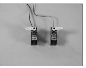
OO 3. Test fit the aileron servo into the pocket in the bottom of the wing. Note that the servo output will face to the front of the aircraft.
