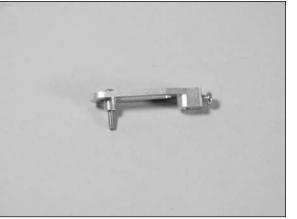
10. Use a #1 Phillips screwdriver to start the screw О in to the outermost hole in the servo arm. Tighten the screw so the brass steering arm bushing is tight against the servo arm.
