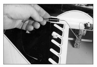
O 9. Connect a 3-inch (76mm) servo extension to the lead on the aileron servo. Tie a piece of string or dental floss around the connection to prevent the two from unplugging accidentally. Install an extension for both aileron servos at this time.
