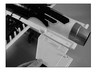
OO 8. Use two 2mm x 12mm self-tapping screws and a #1 Phillips screwdriver to secure the stabilizer to the fuselage. Use care not to over-tighten the screws and cause damage to the fuselage or stabilizer.
