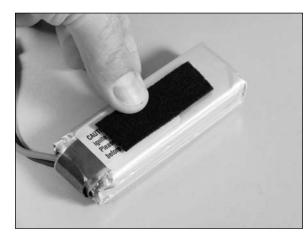
2. Apply the hook and loop tape inside the Ο fuselage in the battery compartment. Use the harder plastic side of the hook and loop tape on the battery.
