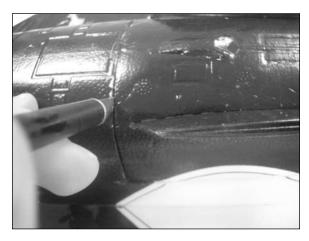
• 2. Use a hobby knife with a #11 blade, or a razor saw with a fine tooth blade, to cut through the glue joint on the front and rear seam lines of the hatch.
