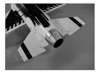
**Note**: The stabilizer tips will be lower than the center of the stabilizer at the fuselage when the fuselage is upright. This is scale for the F-16 and is correct.
