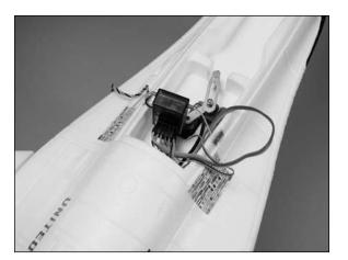
• 5. Use a small piece of hook and loop tape to mount the receiver in the fuselage as shown. The edge of the receiver should be flush with the edge of the cockpit opening as seen in the following step.
