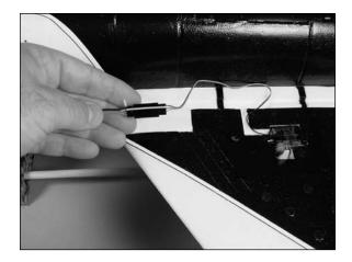
O 10. Carefully lay the extension from the elevator servos into the channel on each side of the fuselage. The aileron extension will than be placed on top of the elevator extension. Both extensions are then inserted into the fuselage where the channel turns to enter the fuselage.
