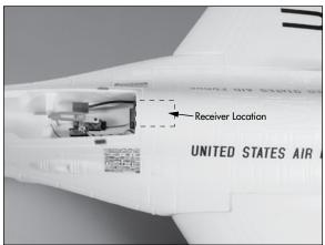
O 6. Use a small piece of hook and loop tape to mount the remote receiver alongside of the steering servo. Make sure the position of the remote receiver will not interfere with the operation of the steering servo when it is installed.
