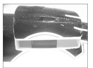
*Note*: When gluing the hatch back in position make sure that the motor wires are routed in the slot on the top of the fuselage. If they are not in this slot the hatch will not seat properly.
