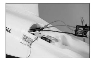
• 2. Apply a small piece of hook and loop tape to the bottom of the speed control.
