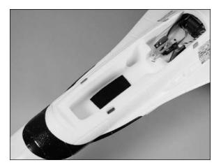
3. Place the battery into the battery compartment in О the fuselage. The battery will be positioned as far back in the compartment as possible to achieve the correct Center of Gravity when you are using the recommended setup.
