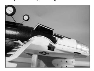
• 3. Repeat Steps 1 and 2 to install the remaining ventral fin on the bottom of the fuselage.
