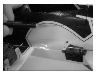
4. Once you are sure that you have cut through the hatch joints all the way around the hatch, use a small amount of force to rock the hatch in a rolling motion side to side. A small amount of movement should break loose the last glue joint on the top of the fan unit and remove the hatch/fan assembly.
