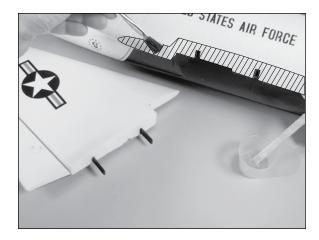
**Note**: You can use a paper towel that has had rubbing alcohol applied to it to remove any excess epoxy from your airframe. Use care not to get the alcohol on the decals as it could damage them.
