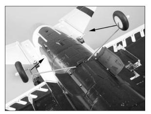
• 5. Lift the canopy hatch from the top of the fuselage. The hatch is held in position using four small magnets and will take a light amount of force to remove.
