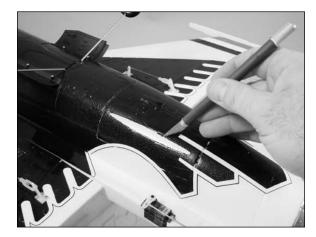
OO 2. Test fit the ventral fin in the slot on the bottom of the fuselage. The taller portion of the fin will face to the front of the fuselage and the decal will face to the wing tip. Once satisfied with the fit remove the fin from the fuselage. Mix a small amount of 6-minute epoxy. Apply the epoxy in the slot and insert the ventral fin in the slot. Allow the epoxy to fully cure before proceeding to the fin installation.
