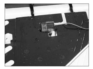
• 5. Repeat Steps 3 and 4 to install the aileron servo in the opposite wing panel.
