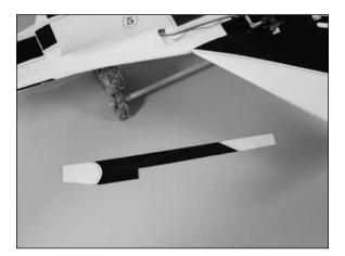
12. Remove the backing from the decal. Starting at the front, hold the rear of the decal up and align the trim scheme from the decal to the scheme on the aircraft. Carefully work toward the rear of the fuselage, pressing the decal down and guiding the extensions under the decal to remain in the channel.
