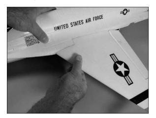
O 4. Fit the remaining wing panel to the fuselage. Stand 6–8 feet (3–4 meters) from the front of the airframe. When viewed from the front, both panels should be flat (parallel) along the bottom to be properly aligned. Use sandpaper to lightly sand the plastic joiner to correct the alignment.
