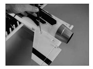
• 9. Repeat Steps 6 through 8 to attach the remaining stabilizer to the fuselage.
