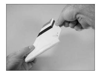
OO 7. Check the fit of the stabilizer to the fuselage. Note that the control horn on the stabilizer will face toward the bottom of the fuselage when the stabilizer is installed.
