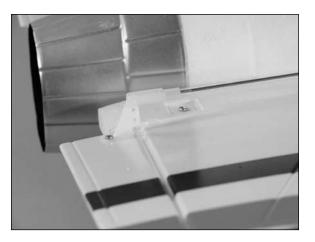
• 15. Repeat Steps 13 and 14 to install the second elevator linkage. The left and right linkages will be mirror images of each other when installed.
