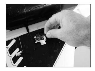
OO 4. Remove the servo and scuff the surface of the servo where it contacts the wing using sandpaper. Clear any residue left from the sanding process using a paper towel and rubbing alcohol. Mix a small amount of 6-minute epoxy. Place a small amount of epoxy in the servo pocket, then install the servo, pressing it into the epoxy. This will keep the servo secure in the wing during the operation of your model.
