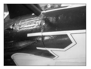
O 3. Using a hobby knife and #11 blade, cut down the side seams of the hatch at approximately a 45-degree angle to the horizontal line of the fuselage.
