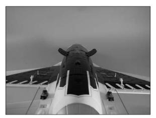
• 3. Use a hobby knife with a #11 blade to remove the decal from the bottom of the fuselage to expose the slot for the main landing gear.
