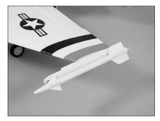
• 4. Repeat Steps 1 through 3 to install the remaining missile to the mount on the opposite wing tip.
