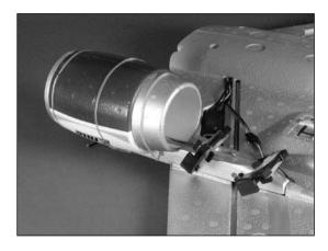
• 9. Tuck the wires neatly into the wire channels. Trim the foam if necessary to fit the connection between the servo and servo extension. Cover the wires using the wiring decal.
