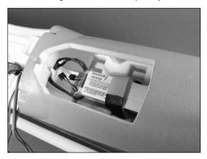
2. Attach the wing to the fuselage using four 3mm x 40mm screws and four 3mm washers. Remember to plug in the aileron and speed controls before installing the screws.
