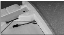
O O 6. Apply the wiring decal over the servo wiring from the engine pod over the servo.
