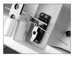
O 7. Use medium CA to glue the pushrod tubes to the pushrod tube support.
