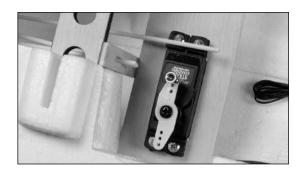
O 6. Slide the elevator pushrod wires through the pushrod connector. Center the elevators and secure the wires using the 3mm setscrew.
