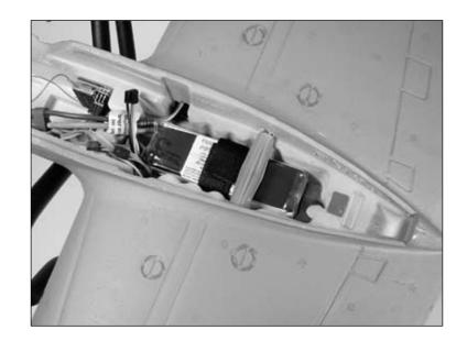
**Note**: When using our recommended Brushed Motor Power System, you MUST use a separate BEC or receiver battery pack to power the radio gear if using more than 3 servos.
