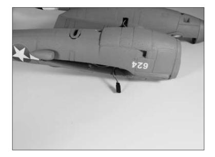
○ ○ 2. Turn on the transmitter and apply power to the receiver. Check that the aileron servo is operating properly. Center the aileron trim and control stick and set any sub-trims to 0. Attach the servo arm to the servo so it is as close to perpendicular as possible when the servo is in the neutral position.
