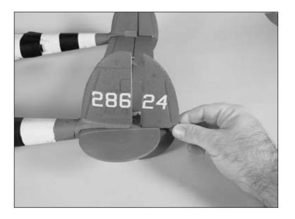
O O 2. Use a hobby knife to cut three slots into the rudder as shown.
