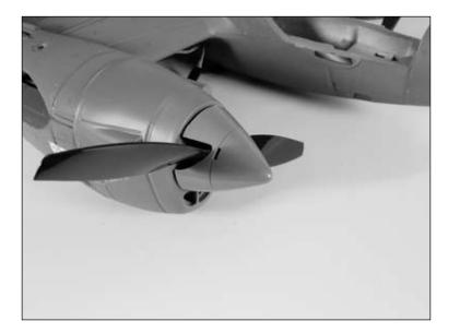
• 10. Repeat Steps 6 through 9 to install the remaining motor. When checking the second motor in Step 4 (without the propeller installed), the motors will rotate opposite directions as shown in the photo.
