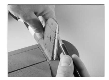
○ ○ 8. Test fit the rudder. Check that it can move freely without binding against the elevator. Trim the rudder or hinge slots in the fin as necessary. Complete the rudder installation by applying foam-safe CA to the hinges and sliding the hinges into the slots in the fin. Be sure to set just enough gap between the fin and rudder to allow free movement of the rudder to the left and right.
