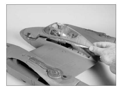
2. Remove the servo cover from the bottom of the left Ο boom by lifting it from the rear.
