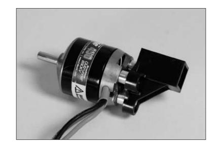
$\bigcirc$   $\bigcirc$  2. Use a razor saw to cut the motor mount stick to a length of  $1 \frac{1}{4}$  in (31mm) for the E-flite Park 450 outrunner motor.
