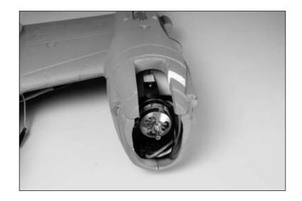
○ ○ 5. Solder both sets of motor leads together with a male EC3 connector. Make sure to solder the positive to positive and negative to negative. Check operation of the motors. The left-hand motor (when viewed from behind) should rotate counterclockwise when viewed from the front. The right-hand motor (when viewed from behind) should rotate clockwise when viewed from the front.
