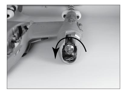
**Note**: If either motor is running in the opposite direction that it should, simply reverse any two of the wire leads that connect to the ESC.
