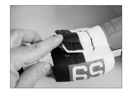
3. Locate a  $10^{3}/_{4}$  in (273mm) pushrod wire and remove the clevis. Slide the wire into the pre-installed tube in the Ο fuselage threaded end first. The correct tube will exit near the elevator control horn.
