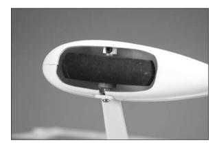
20. Repeat steps 14 through 19 to install the remaining main wheel and wheel pant.
