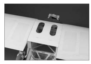
5. Separate the elevator and stabilizer. The hinges have been pre-glued into the elevator, so check them, but do not attempt to remove them.
