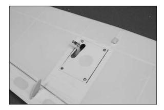
20 15. With the aileron servo centered, attach the Z-bend of the pushrod to the control horn.
