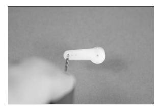
2. Attach the pushrod connector to the outside hole of the steering arm as shown. The washers that come on the connector are not needed and can be removed. Tighten the nut so it is secure on the steering arm but is not tight. There should be a small amount of play between the arm and the connector and the connector should be able to rotate freely on the arm.
