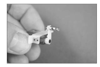
4. Use a very small amount of medium CA on a toothpick to secure the nut to the bottom of the connector threads. Do not use thin CA for this step as it can wick through the nut and glue the connector to the arm. Make sure the connector still rotates freely in the arm after the glue is cured.
