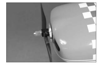
8. Use a 6mm open-end wrench to tighten the nut, securing the assembly to the motor shaft. Check that the backplate does not rub against the cowl. If it does, loosen the nut, move the assembly forward, then re-tighten the nut.
