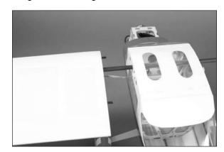
4. Slide the wing so it fits tightly against the fuselage.
