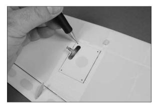
11. Use a pin vise and 1/16-inch (1.5mm) drill bit to drill four holes for the mounting screws. Use care not to accidentally puncture the covering on the top of the wing or to push too hard on the mounting rails, as this could break them.
