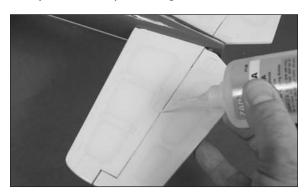
17. Check that the hinges are secure by gently pulling on the control surface. If not, apply thin CA to any hinges that are not glued and recheck.
