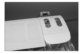
O 5. Place the remaining wing panel into position.
