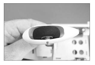
O 23. Use canopy glue to glue the nose gear wire into the recess of the wheel pant. Use low-tack tape to hold the wheel pant in position while the glue cures. Allow the glue to fully cure before proceeding.
