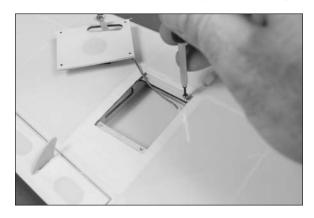
13. Apply 2-3 drops of thin CA in each of the holes to harden the surrounding wood. This will harden the threads so the screws do not easily strip the surrounding wood.
