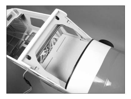
3. Remove the backing from the adhesive strips on the bottom of the seat backs. Attach the seat backs to the forward cockpit floor.
