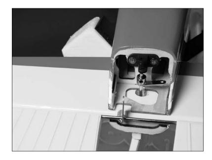
**Note**: It is very important to use threadlock to ensure this assembly does not come apart during flight.
