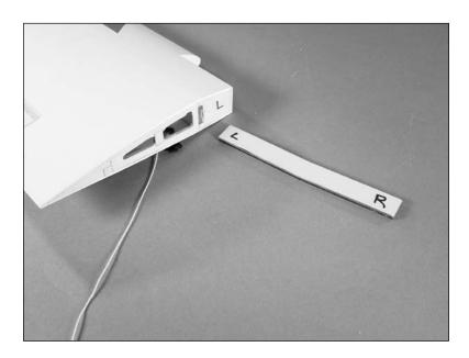
2. Slide the wing joiner into the wing panel. Use a pencil to mark the joiner against the wing. The joiner should fit snug in the wing. If it does not fit, lightly sand the joiner until it does fit nicely.
