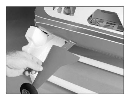
2. Secure the left half of the landing gear using two 6-32 x 3/8-inch socket head screws and two #6 washers. Use a 7/64-inch ball driver to tighten the screws.
