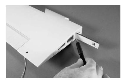
3. Slide the joiner into the opposite wing panel. It should slide in to slightly hide the line drawn in the previous step. If not, lightly sand the ends of the joiner until it fits equally into both wing panels.
