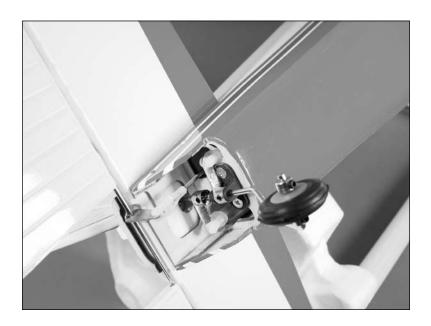
17. After centering the tail wheel, tighten the 3mm setscrew to secure the pushrod. Use this connection to trim the steering of your Beaver on the ground. DO NOT use the radio trim to correct the steering trim.
