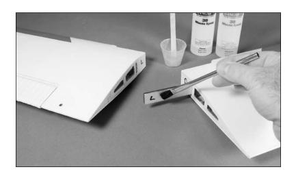
7. Use low-tack tape to hold the two wing panels tightly together until the epoxy fully cures.
