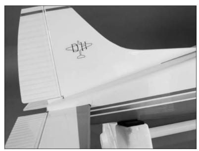
O 11. Use a felt-tipped pen to trace the outline of the fuselage onto the fin. Also trace the outline of the dorsal fin onto the top of the fuselage.
