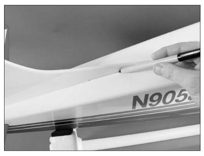
O 12. Use a sharp hobby knife to cut the covering slightly below the lines drawn. Be very careful not to cut into the underlying wood, as this will weaken the fin and cause it to fail in flight. Also trim the covering on the top of the fuselage.
