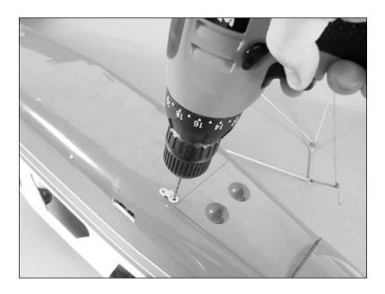
4. Attach the float mount to the bottom of the fuselage using two straps, four 3mm x 12mm sheet metal screws and a #2 Phillips screwdriver.
