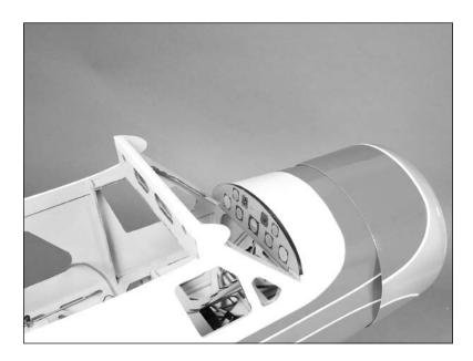
2. Test fit the forward cockpit floor in the fuselage. Trim the floor as necessary using hobby scissors. The cockpit floor is then glued in using medium CA.
