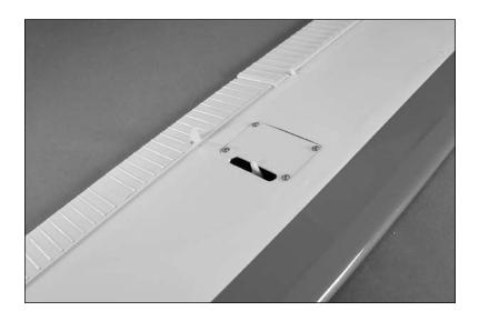
11. Slide the bend of the 2<sup>3</sup>/<sub>16</sub>-inch (56mm) pushrod into the hole of the aileron servo. Secure the pushrod using the pushrod connector.
