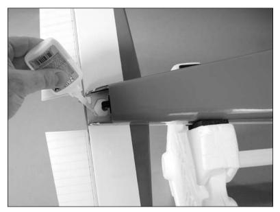
O 10. Insert the rudder control rod into the fuselage, then slide the fin into the slot in the top of the fuselage.
