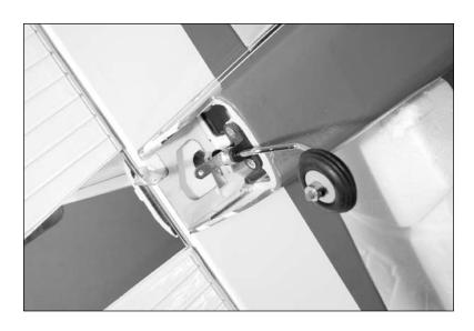
13. Slide the pushrod into the hole in the servo horn and secure it using a pushrod connector.
