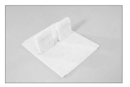
O 10. Secure the rear cockpit floor in the fuselage using four #2 x 3/8-inch sheet metal screws. The screws will go through the rear cockpit floor and into the block installed in Step 8. Route the leads for the flaps and ailerons from underneath the floor at this time.
