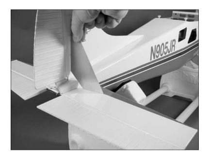
14. Slide the fin up slightly so the rudder control horn can be installed on the rudder control rod. Use a setscrew and the provided hex wrench to tighten the setscrew on the flat area of the control rod. Note that the tab on the horn faces toward the top of the fuselage when installed.
