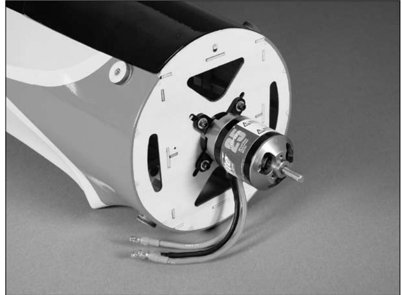
**Note:** The blind nuts in the fuselage for mounting the motor can be positioned for a variety of motors. Position them so they are aligned with your particular motor before mounting it to the firewall.
