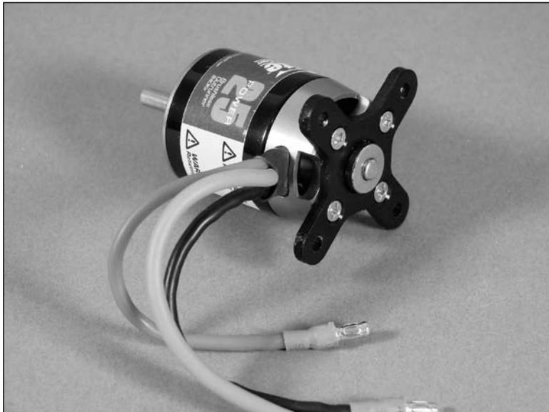
2. Attach the motor to the firewall using four 4-40 x 1/2-inch socket head screws, four #4 washers and a 3/32-inch ball driver. Make sure to use threadlock on the four screws to prevent them from vibrating loose.
