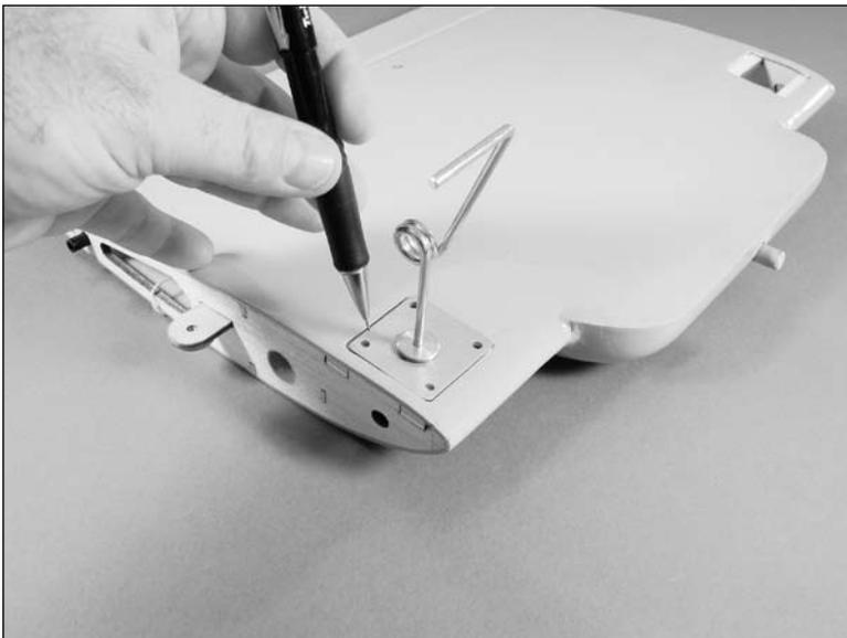
2. Use a drill and 5/64-inch (2mm) drill bit to drill the four holes for the mounting screws. Use care not to accidentally drill through the top of the wing.
