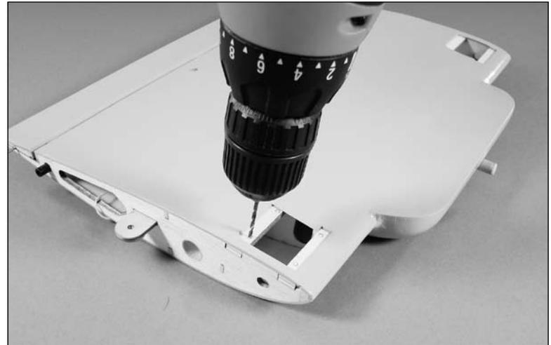
3. Apply a few drops of thin CA to each of the holes to harden the surrounding wood.
