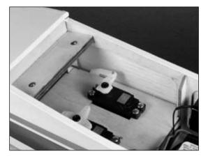
**Note**: Use side cutters to trim down the excess pushrod wire and remove the extra arms from the servo horn.
