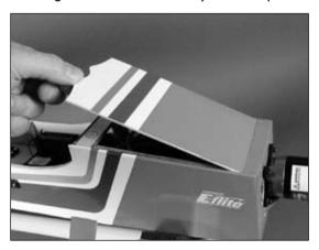
○ 4. Plug in the aileron (and flap) servo leads. Slide the wing dowels into the holes at the front. Use the two 6-32 x 1" socket head screws and two #6 washers to secure the wing.
