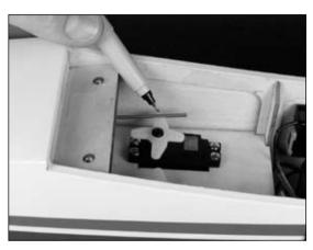
○ 5. Bend the pushrod wire at the mark made in the previous step. Enlarge the hole in the servo arm using a 5/64" (2mm) drill bit. Secure the pushrod wire to the servo horn using a pushrod connector.
