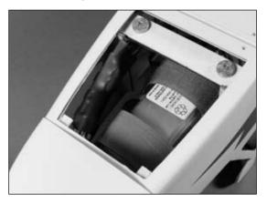
**Note**: Now would be a good time to plug the speed control into the receiver and check the operation of the motor. It should rotate counterclockwise when viewed from the front of the fuselage. Once the operation of the motor has been checked, unplug the battery and attach the battery hatch.
