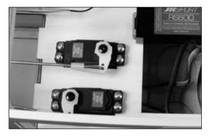
**Note**: Ensure the radio is turned on with the trims and sub-trims centered and the servos are centered.
