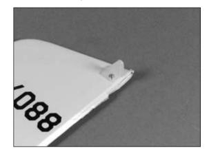
O 10. Roughen the tail gear wire with sandpaper. Use 6-minute epoxy on the tail gear wire to glue into the rudder. • 11. Remove the T-pins from the hinges and use thin CA to glue them in place. Allow the epoxy and CA to cure before continuing to the next step.
