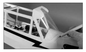
**O** 2. Lightly sand the fuselage inside the line drawn in the last step. Also sand the inside edge of the windshield where it will attach to the fuselage.
