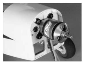
**Note**: The firewall has been prepared to mount the E-flite<sup>™</sup> Power 25 brushless motor. It may be necessary to remove the blind nuts and drill new mounting holes for other motor choices. • 3. Attach the motor to the speed control. Secure the speed control in the fuselage using hook and loop material so it will not move during flight.
