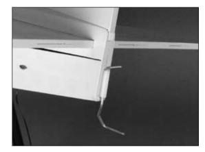
O 3. Drill a 3/32" (2.5mm) hole into the rudder 1<sup>1</sup>/<sub>16</sub>" (27mm) up from the bottom of the rudder. Verify this measurement by holding the rudder in position against the fuselage.
