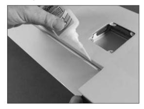
**Note**: Do not use accelerator in the hinging process. The CA must be allowed to soak into each hinge naturally.
