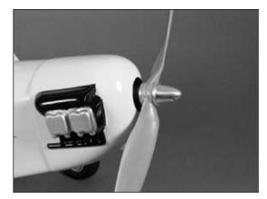
O 6. Position the cowling so it lines up with the propeller and adapter. Allow for 1/8" (3mm) clearance between the propeller and cowl. Drill four 1/16" (1.5mm) holes for the cowl mounting screws. Enlarge the holes in the cowling only using a 1/8" (3mm) drill bit. Secure the cowling using four 2mm x 10mm sheet metal screws.
