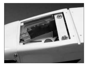
**Note**: Ensure you mount the speed control with the label towards the fuselage sidewall. This will assure maximum cooling for the speed control.
