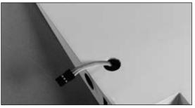
**Note**: A weight tied to a string can be used first, then tied to the servo lead to pull it through.
