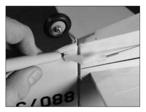
○ 9. Remove the rudder and drill the two locations using a 5/64" (2mm) drill. Mount the horn using two 2mm x 12mm screws and the control horn backplate.
