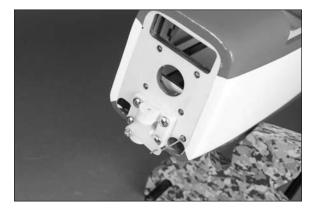
• 4. Use a flat file to make a 1/4-inch (6mm) wide flat on the bottom of the nose gear wire. This will provide a place to tighten the setscrew when the wheel collar is installed.
