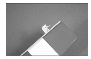
OO 5. Slide the aileron back into position. Center the aileron so the gap at the ends is equal.
