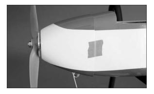
O 5. Measure 3/16-inch (5mm) forward of the edge of the cowl, and in 3/16-inch (5mm) from the paint lines on the cowl. Use a pin vise with a 1/16-inch (1.5mm) drill bit to drill four holes through the cowling and fuselage side for the cowl mounting screws.
