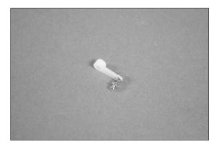
OO 4. Connect a 6-inch (152mm) servo extension to the servo lead. Use string of dental floss to secure the leads so they do not accidentally disconnect inside the wing. Use a #O Phillips screwdriver to remove the servo horn from the servo.
