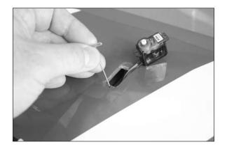
OO 7. Use a #1 Phillips screwdriver to thread a servo mounting screw into each of the holes to cut threads in the surrounding wood. Remove the screw before moving to the next step.
