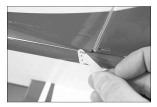
OO 9. Insert the control horn in the slit in the rudder (or elevator).
