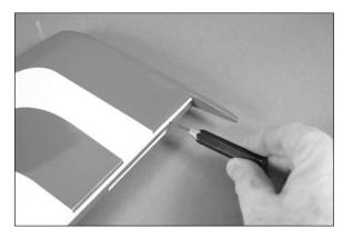
OO 2. Use a pin vise and 1/16-inch (1.5mm) drill bit to drill a hole in the center of each hinge slot in the aileron to create a tunnel for the CA to wick into. This will allow the CA to penetrate the hinge, creating a better bond between the hinge and surrounding wood.
