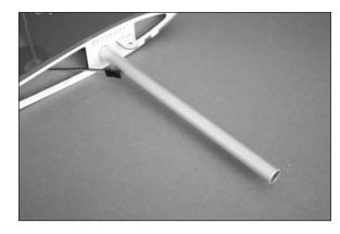
• 2. Slide the tube into the socket in the fuselage. Make sure to guide the lead for the aileron servo in the fuselage when positioning the wing.
