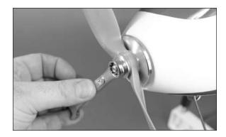
• 11. Place the spinner cone on the propeller. Use the screw included with the spinner assembly and a 2.5mm hex wrench to secure the cone in position.
