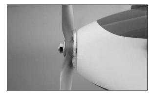
• 4. Use low-tack tape to hold the cowling in position for the following step. Make sure the propeller can rotate without the backplate rubbing against the cowling.
