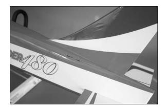
• 2. Use a felt-tipped pen to trace the outline of the fuselage on the bottom of the fin.
