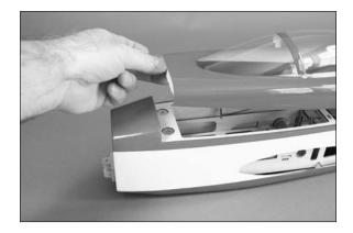
2. Use a #1 Phillips screwdriver to thread a servo mounting screw into each of the holes to cut threads in the surrounding wood. Remove the screw before moving to the next step. Prepare all four mounting holes at this time.
