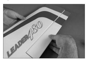
OO 8. Move the aileron through its range of motion several times to break in the hinges. This will reduce the initial load on the servo during your first flights.
