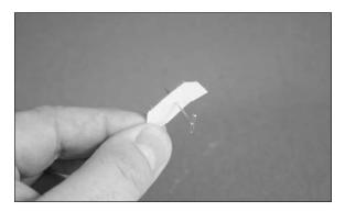
OO 3. Insert the hinges in the rudder (or elevator). The T-pin will rest on the edge of the bevel of the control surface.
