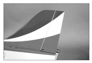
OO 5. Saturate each hinge with thin CA. Apply CA to both side of the hinge.
