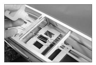
○○ 4. Secure the elevator servo in the fuselage using the screws provided with the servo and a #1 Phillips screwdriver. The output shaft of the servo faces the rear of the fuselage when installed. Remove the servo horn from the servo using a #0 Phillips screwdriver.
