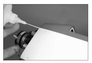
9. Once the CA has cured, use four #0 Phillips head wood screws and a #1 Phillips screwdriver to secure the cowl to the fuselage.
