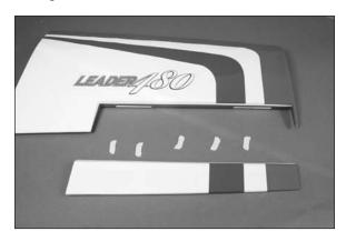
OO 2. Use a pin vise and 1/16-inch (1.5mm) drill bit to drill a hole in the center of each hinge slot in the wing to create a tunnel for the CA to wick into. This will allow the CA to penetrate the hinge, creating a better bond between the hinge and surrounding wood.
