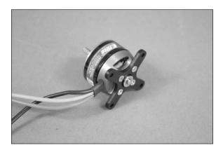
2. Secure the motor to the firewall using the four 18mm aluminum motor standoffs, four 3mm x 30mm socket head cap screws, four 3mm washers and four 3mm lock washers. Use a 2.5mm hex wrench to tighten the screws. Make sure to use threadlock on these screws as well to prevent them from vibrating loose.
