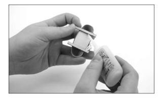
• 5. Use a hobby knife and #11 blade to remove the covering from the canopy. Test fit the pilot into the canopy. It may be necessary to lightly sand to opening to fit the pilot.
