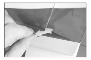
OO 10. Slide the control horn backplate over the end of the control horn from the opposite side of the control surface. Snap the backplate so the horn is held tightly in position. Apply 2–3 drops of thin CA to the backplate where it contacts the control horn to keep it from accidentally coming loose in flight.
