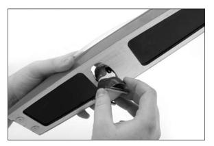
• 6. Once satisfied with the fit, use medium CA to glue the pilot in the canopy. Apply the glue to the stiffeners to keep the pilot in the canopy.
