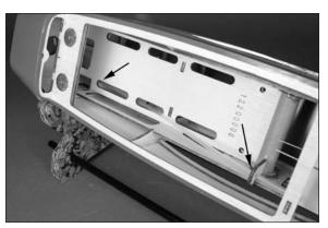
• 2. Insert the Z-bend of the pushrod wire into the nose gear steering arm as shown.
