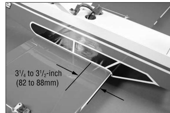
When balancing your Alpha 450 Sport 450, support the plane upright at the marks made on the bottom of the wing with your fingers or a commercially available balancing stand. Move the motor battery as necessary so the model hangs level or slightly nose down. This is the correct balance point for your model.
