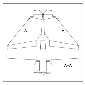
• 4. View the airframe from the rear and make sure the wing and stab are parallel. If not, lightly sand the stab saddle until they are.
