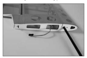
2. Remove the hatch from the fuselage. Slide the wing panel with tube into position on the fuselage.
