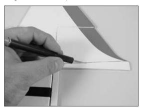
• 4. Position the fin back onto the fuselage. Use a square to check the alignment between the fin and stabilizer. Lightly sand the bottom of the fin until the alignment is correct.
