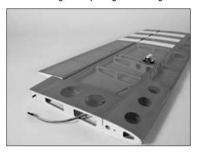
OO 3. Secure the aileron servo using the screws provided with the servo.
