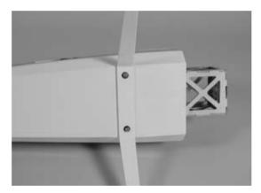
○ 2. Slide the 4-40 x 1" machine screw through one of the 1³/₄" wheels. Slide a #4 steel washer so it fits against the wheel. Next secure a 4-40 nut against the washer. Make sure the wheel still spins freely. Slide a second #4 steel washer onto the bolt. This washer will fit inside the wheel pant.
