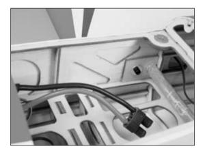
• 4. Test fit the wing fairing (filets) into position against the wing. You may need to loosen the screw holding the wing in place to install the fairing. Installing the fairing now will guarantee that it lines up correctly with the holes in the fuselage.
