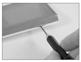
O 2. Slide three hinges into the slits in the aileron. Center the slot in the hinge with the hole drilled in Step 1. Place a T-pin in each hinge to prevent it from being pushed into the wing when installing the aileron.
