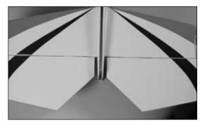
O 3. Measure from the stab tip to the wing tip. Adjust the stab until the measurements are equal.
