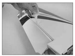
○ 4. Firmly grasp the wing and aileron and gently pull on the aileron to ensure the hinges are secure and cannot be pulled apart. Use caution when gripping the wing and aileron to avoid crushing the structure.
