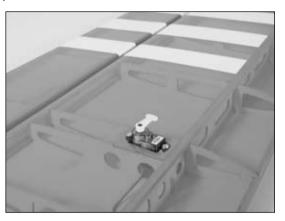
O 4. Use a hobby knife to enlarge the inboard hole in the control horn to fit the 4" (100mm) long aileron pushrod wire.
