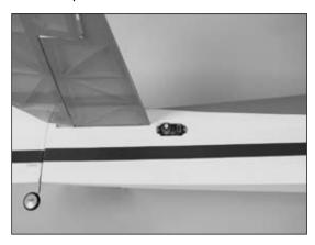
O 2. Use a hobby knife to enlarge the inboard hole in one of the remaining control horns. Attach the 4<sup>1</sup>/<sub>2</sub>" (115mm) pushrod wire to the control horn. ○ 3. Attach the micro control horn to the elevator using the control horn backplate and 6-minute epoxy.
