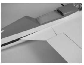
○ 5. Use 6-minute epoxy to glue the fairing to the wing. Make sure not to get glue on the fuselage. Use tape to hold the fairing tight against the wing while the epoxy cures.
