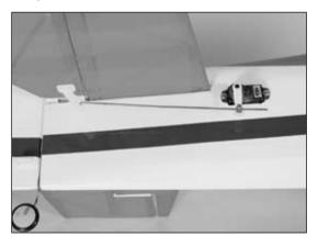
O 5. Repeat Steps 1 through 4 for the rudder servo and linkage using the 5<sup>3</sup>/<sub>4</sub>" (145mm) pushrod wire.
