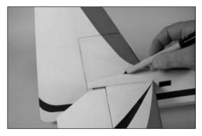
O 3. Remove the covering from the bottom of the fin using the same technique used for the stabilizer.
