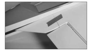
**Note**: The fairing may not fit tight against the fuselage at this time. This will be addressed once both fairings have been installed.
