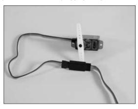
**Note**: We suggest using the long 3D servo arms for the Mini FuntanaX. Replace all existing arms before installing the servos.
