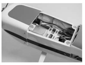
**Note**: Place a piece of hook and loop tape on the bottom of the battery and on the fuselage where the battery rests. This will keep the battery from shifting forward or backward during extreme maneuvers. 6. Install the battery hatch to the top of the fuselage.
