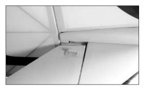
○ 4. Install the micro control connector onto the elevator servo arm. Pass the elevator pushrod wire through the connector. With the radio on and elevator trim centered, center the elevator. Secure the elevator pushrod wire using the 2mm x 4mm screw and a small Phillips screwdriver.
