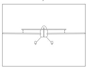
O 5. Double-check the adjustments from Steps 1 through 3. Use a felt-tipped pen to trace the outline of the fuselage onto the top and bottom of the stabilizer.
