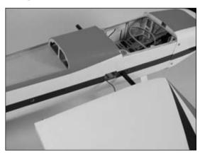
○ 3. Slide the remaining wing panel into position. Secure the panels using 4-40 x 1/2" machine screws with #4 washers (silver) using a 3/32" hex wrench.
