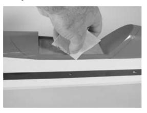
4. Use Formula 560 canopy glue to glue the canopy to the fuselage. Use masking tape to hold the canopy in position until the glue fully cures.
