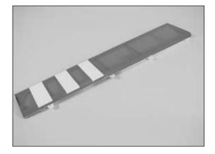
**Note**: Do not use CA accelerator during the hinging process. The CA must be allowed to soak into the hinge to provide the best bond. Using accelerator will not provide enough time for this process.
