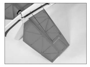
**Note**: Make sure the rods are positioned so they don't interfere with the operation of the rudder and elevator linkages.
