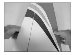
O 5. Work the aileron up and down several times to work in the hinges and check for proper movement.
