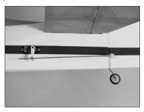
O 6. Attach the carbon stabilizer supports between the fuselage and stabilizer. Make notches in the stabilizer and fuselage for the rods to rest in. Secure the rods using 6-minute epoxy.
