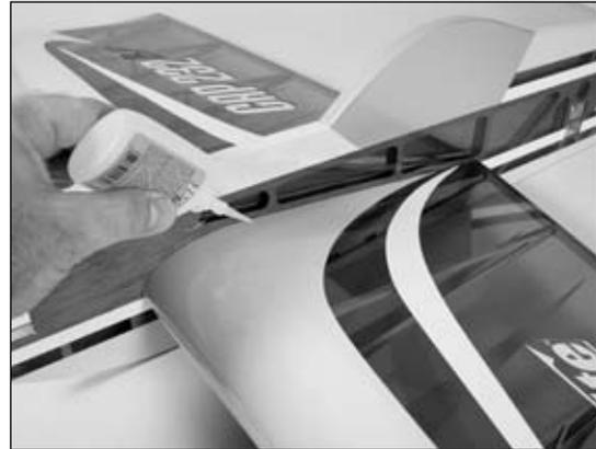
**Note:** Avoid using a CA accelerator to allow the CA to wick well into the wood of the fuselage and wing. This will provide the best bond between the two items.
