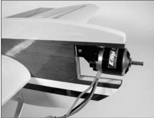
**Note:** Check that your motor has right thrust. The motor will be angled towards the right when viewed from the top of the aircraft as shown.
