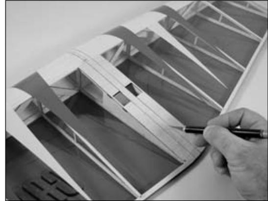
**Important:** Do not cut into the underlying wood. This will weaken the structure and could cause failure in flight. As an option, you can use a soldering iron or hot knife with light pressure to carefully melt the covering and avoid the potential of cutting into the wood.
