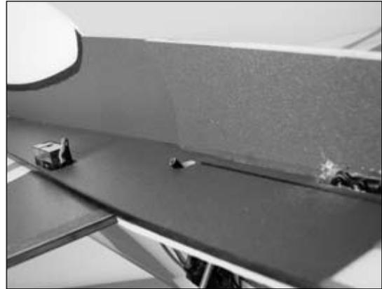
**Hint:** You can just drop the disks into position and check to make sure the strut extends beyond the disk instead of measuring it.
