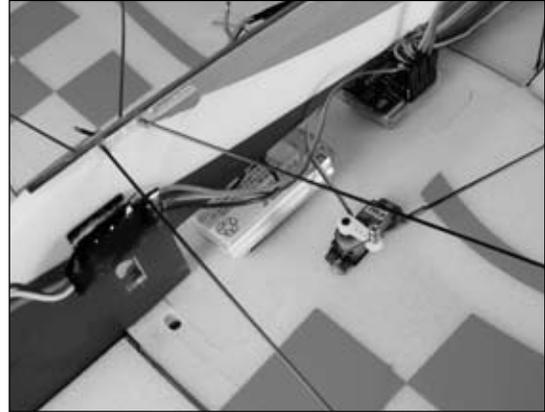
**Note:** It is suggested to secure the motor wires to the fuselage to prevent them from coming in contact with the propeller or servos when performing extreme maneuvers.
