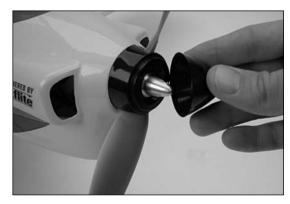
• 7. Insert the 'hex to round' adapter onto the shaft. Then, slide the 6mm washer included with your gearbox onto the output shaft.
