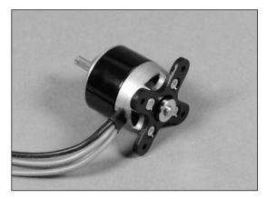
○ 2. Using four 4-40 x 43mm socket head screws and washers and outrunner offset spacers, attach the motor with X-mount to the blind nuts on the firewall The offset spacers have already been sized correctly so you have proper clearance when the cowling is installed later.
