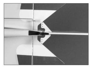
**Note**: The control horn has ears that will allow it to only slide into the rudder from one direction. These ears rest against the side of the rudder when installed correctly.
