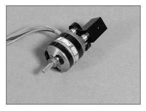
3. First, cut 3/16" inches (5mm) off the end of the included Firewall Stick Mount so the motor properly clears the cowling. Assemble the Outrunner stick mount to the Park 480 Outrunner using the spacers and screws provided with the mount. Attach to the Brio firewall using the four 4-40 x 1/2" socket head bolts. Attach the motor to the Firewall Stick Mount as shown.
