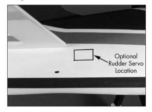
At this time, we suggest that you trial fit the battery and receiver into the front of the fuselage and follow the steps outlined on page 49 and check the CG location. If it is nose heavy, you might consider installing the servo at the optional rear location. If you do not anticipate an issue, than proceed with Step 4 and install the rudder servo in the fuse for a pull-pull system.
