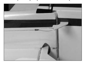
7. Slide the micro cable adjust connector into the micro control connector and use a 2mm x 3mm screw to hold it in position. Repeat Step 7, installing the cable through the cable connector.
