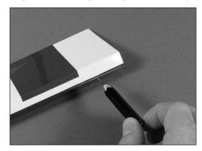
○ 2. Slide three hinges into the slits in the aileron. Center the slot in the hinge with the hole drilled in Step 1. Place a T-pin in each hinge to prevent it from being pushed into the wing when installing the aileron.
