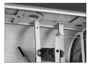
8. The cables will cross inside the fuselage to get the proper geometry for the rudder to operate correctly.
