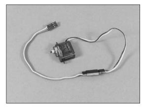
O 3. Place the servo in the wing. Guide the servo lead out through the opening at the wing root.
