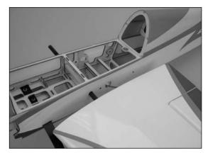
○ 3. Slide a #4 washer onto a 4-40 x 1/2" socket head screw. Slide the remaining wing panel into position. Secure the panels using 4-40 x 1/2" socket head screws with #4 washers (silver) using a 3/32" hex wrench.
