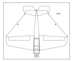
○ 5. View the airframe from the rear and make sure the wing and stab are parallel. If not, lightly sand the stab saddle until they are.
