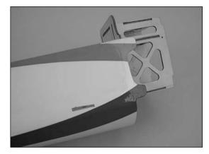
○ 2. Slide the landing gear into the fuselage. The holes in the gear will only line up when installed correctly. Slide a #4 washer onto each of the four 4-40 x 1/2" socket head screw. Place a drop of threadlock onto each of the 4-40 screws. Slide the screws through the landing gear and into the pre-installed blind nuts. Use a 3/32" hex wrench to tighten each of the screws.
