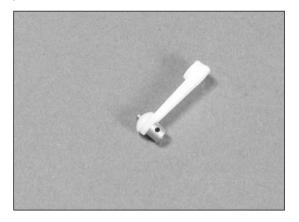
○ 6. Turn on the radio system and center the aileron trim and stick. Make sure the aileron servo is operating properly using the transmitter. Slide the pushrod wire through the micro connector. Install the servo arm parallel to the aileron hinge line. Center the aileron, and secure the position of the wire using the 2mm x 4mm screw and a Phillips screwdriver.
