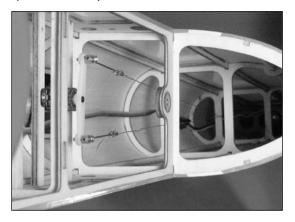
O 9. Remove the tape from the control surface. Install the second cable following Steps 9 through 11. Tension the cables lightly using the cable connectors to pull the surface into neutral.
