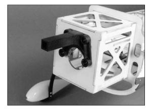
O 2. Attach the outrunner motor to the outrunner motor mount using the included spacers (4) and 3mm x 8mm screws (4).
