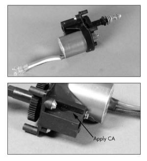
*Hint*: The gearbox is in two pieces. Apply a bead of medium CA where the two pieces join to stiffen the mount for extreme aerobatics.
