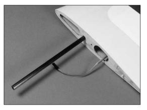
**O** 2. Remove the hatch from the fuselage. Slide the wing panel with tube into position on the fuselage.
