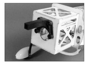
A. Slide the gearbox into position on the motor mount. Use a 1/16" (1.5mm) drill to drill a hole on each side of the gearbox and into the mount. Stagger the holes so the screws will not interfere with each other. Secure the gearbox using three #2 x 8mm screws.
