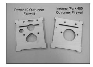
○ 2. Attach the firewall to the sub-firewall structure on the front of the fuselage nose at this time using 6-minute epoxy or thick CA. Epoxy is best for this application. Make sure all joints are secure when finished so the firewall does not detach from the sub-firewall.
