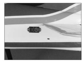
• 2. Attach the micro control horn to the elevator using a micro control horn backplate. Apply a few drops of medium CA to the backplate.
