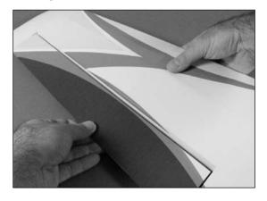
○ ○ 5. Work the aileron up and down several times to work in the hinges and check for proper movement.
