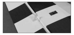
O O 2. Attach a 6" servo extension to the aileron servo. Secure the extension using string or a commercially available clip.
