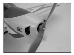
**Note**: Two spacers have been provided that are placed between the propeller and spinner backplate. Use the thin spacer for low-pitch propellers, the thick spacer for high-pitch propellers. This will prevent the blades of the propeller from contacting the spinner backplate.
