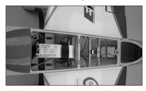
*Hint*: It is recommended you may use a piece of hook and loop strapping around the battery to help secure it in position.
