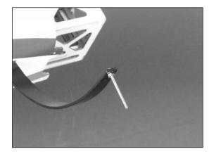
○ ○ 4. Thread a 2mm nut 1/8" (3mm) from the first nut. Use threadlock or thin CA to keep the nut from rotating. Slide the wheel on and thread a final 2mm nut onto the screw, using threadlock or thin CA to keep the nut from rotating.
