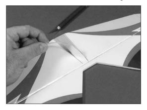
**Note**: You can use a soldering iron or hot knife instead of a regular old hobby knife. This will help in reducing the chance of damaging the wood.  O 8. Slide the stab and elevator back into position. Again, check the alignment and make sure everything lines up. Wick Thin CA into the joint between the fuselage and stabilizer. Make sure to glue both top and bottom. Do not use accelerator−allow the CA to wick in as far as possible, providing the best bond.
