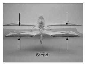
• 6. Double-check the adjustments from Steps 1 through 3. Use a felt-tipped pen to trace the outline of the fuselage onto the top and bottom of the stabilizer.
