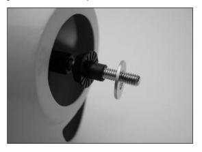
O 8. Slide the propeller onto the gearbox shaft. Slide the spacer included with the spinner onto the gearbox shaft in front of the prop as needed.
