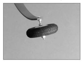
**Note**: Be very careful when using thin CA as not to glue the wheel so it won't rotate on the 2mm x 25mm screw.
