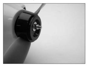
O 10. Snap the spinner cone onto the spinner backplate.
