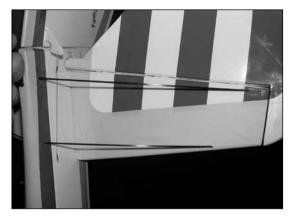
○ 10. Attach the rudder using three CA hinges. Use the technique as described in Aileron Hinging for this procedure.
