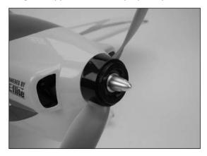
**Note**: It is very important that you check to be sure the propeller is balanced before installing onto the shaft. An unbalanced propeller will cause performance issues. Some propellers will need the center hole drilled out to fit the shaft size of your outrunner. It is very important the hole is drilled concentric or it can cause the propeller to be unbalanced.
