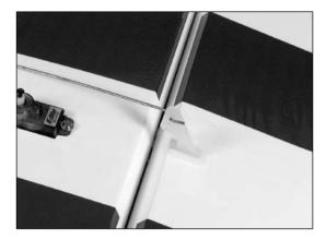
O 5. Attach the micro control connector to a long 3D servo arm. Be sure to use the included retainer to secure the micro control connector to the servo arm. Remove the remaining unused part of the servo arm.
