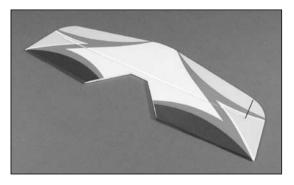
**O** 2. Cut the rear of the fuselage using a hobby knife to allow the stabilizer to be slid into the fuselage.
