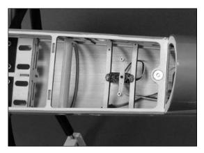
○ 6. Use tape to hold the rudder in neutral. Slide a cable crimp onto the control cable. The cable then goes through the horn, then back through the crimp twice. Pull the wire tight, and then use pliers to secure the crimp. Add a small drop of thin CA inside the brass crimp to help secure the wire. Wipe away any excess immediately.
