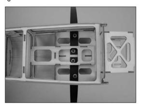
O 3. Slide the 2mm x 25mm bolt through the landing gear. Secure the bolt using a 2mm nut and threadlock.
