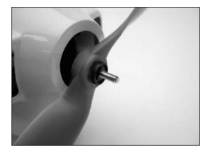
**Note**: Two spacers have been provided that are placed between the propeller and spinner backplate. Use the thin spacer for low-pitch propellers, the thick spacer for high-pitch propellers. This will prevent the blades of the propeller from contacting the spinner backplate.  O 9. Slide the spinner backplate onto the gearbox shaft. Secure the propeller and spinner backplate using a 4mm washer and 4mm locknut. Make sure not to over-tighten the 4mm locknut.
