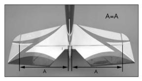
O 4. Measure from the stab tip to the wing tip. Adjust the stab until the measurements are equal.
