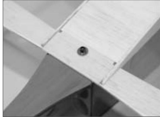
**Note:** The 4-40 socket head screw uses the 3/32" hex wrench.
