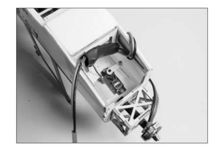
O O 4. Slide the elevator pushrod wire through the center hole in the control horn. Place a small bend in the pushrod wire to apply light tension to keep the pushrod wire from popping out of the horn.
