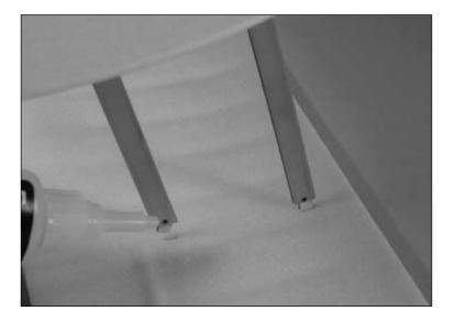
○ ○ 9. Locate the inner struts. Select a front and rear strut. The rear strut has a greater angle than the front as shown in the photo below.
