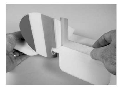
Q Q 2. Slide a micro control horn into the slot in the elevator from the bottom.
