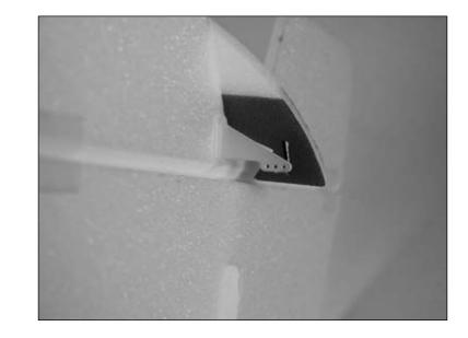
O O 3. Slide the micro control horn backplate onto the control horn from the opposite side of the elevator as the horn. Apply a few drops of foam-safe CA onto the backplate to secure it to the horn.
