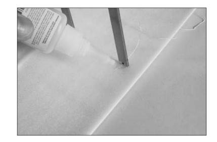
○ ○ 5. Apply very light tension to the rigging thread and apply foam-safe CA to the thread to attach it to the strut. Use scissors to cut the rigging thread once the CA cures.
