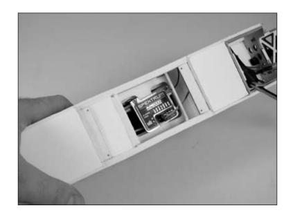
10. Turn on the transmitter and bring the throttle trim and stick to the low throttle position. Plug the battery into the speed control and check the operation of the motor. It should rotate counterclockwise when viewed from the front of the aircraft. Use the instructions provided with your ESC to make corrections to the direction of rotation of the motor if necessary.
