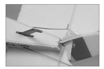
○ ○ 5. Check to make sure the elevator and stabilizer are parallel.
