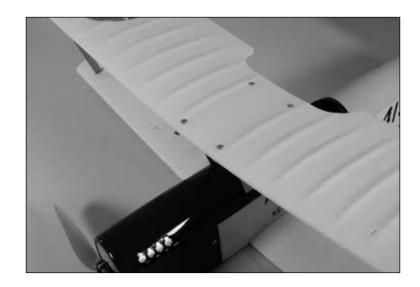
**Note**: The alignment of the wings is **very** important for smooth, predictable flight. Take your time during the next few steps to ensure you do not build a warp into the wing platform at any time.
