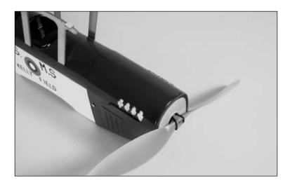
• 9. Use hook and loop tape to secure the battery inside the cowl. The battery can be moved forward or backward to adjust the Center of Gravity.
