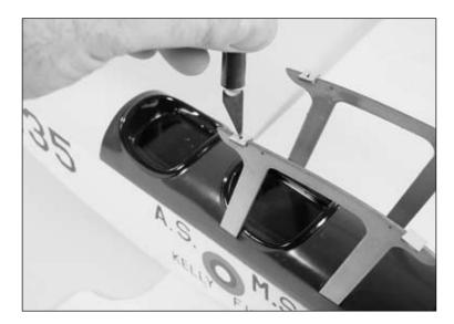
• 4. Use a felt-tipped pen to mark the holes made in the previous step. This will help in sighting the holes through the wing.
