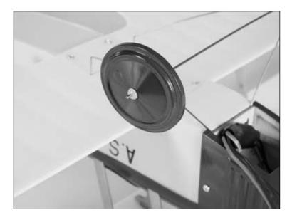
*Hint*: Use medium foam-safe CA on the retainer if it is not snug on the axle. Use care not to glue the wheel to the axle.
