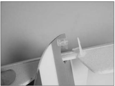
*Note*: The rudder horn is opposite the elevator horn.
