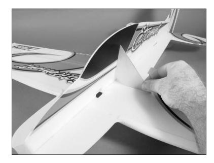
**Note**: Use low-tack tape to tape the control surfaces in their neutral positions. This will make the airframe easier to handle during assembly. Be careful not to tape the printed surfaces as there is a chance of the printing coming off when removing the tape.
