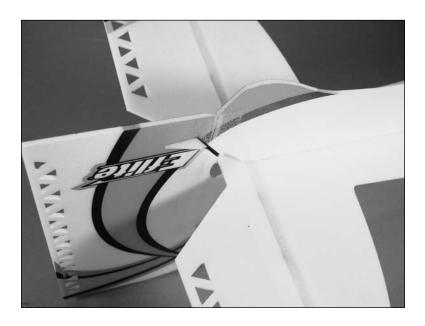
4. Plug the servos into the radio system and make sure they operate and are centered as well. Also center the trims on the transmitter at this time. If you are using a computer radio, start with a clear model program and check that all sub trims are set to 0 and all throws are set to 100%. Prepare the servos for installation by attaching the long 3D arms on the servos and by removing any unnecessary arms from the elevator and rudder servo horns as shown.
