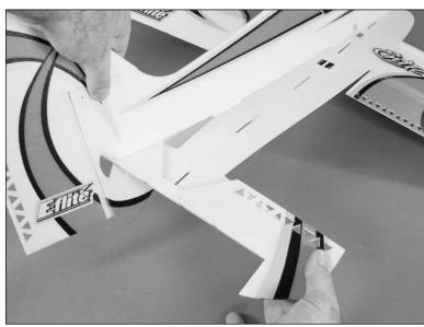
3. Flip the elevator back into its correct position and align the tabs from the vertical fuselage into the slots in the horizontal fuselage. Do not glue the vertical fuse to the horizontal fuse at this time.
