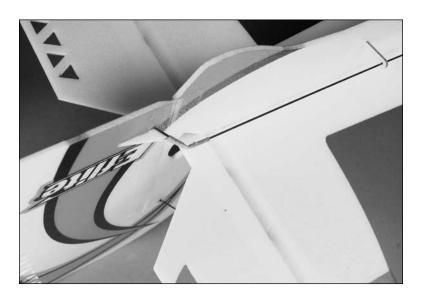
14. Use foam-safe CA to glue the pushrod supports in the notches in the fuselage. Make sure to position the supports so they do not bind the pushrod when operating the rudder.
