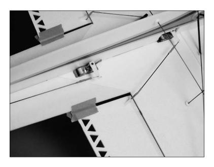
22 13. Repeat Steps 8 and 9 to attach the pushrod to the control horn.
