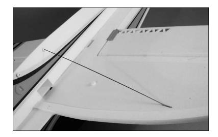
3. Locate the 11 ½-inch (294mm) carbon rod. Position the rod from the slot near the aileron hinge line of the wing to the forward position on the vertical fuselage. Glue ONLY the position at the wing at this time.
