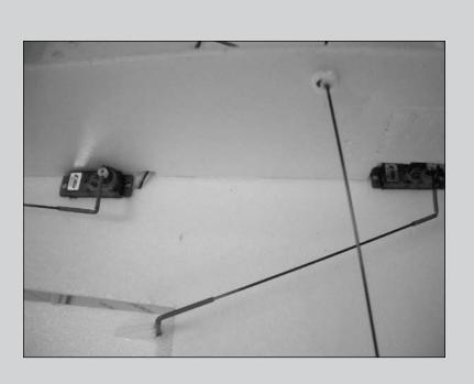
5. Use low-temperature hot glue to secure the servos in the fuselage. All the output arms for the servos will face the front of the aircraft.
