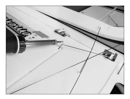
**Note**: You must use a soldering iron to shrink the tubing. The heat from other methods cannot be controlled as well and will cause damage to your airframe.
