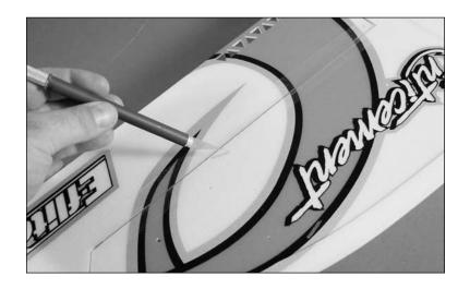
2. Locate the 10<sup>3</sup>/<sub>4</sub>-inch (274mm) carbon rod. Position the rod from the slot near the leading edge of the wing to the rear position on the vertical fuselage. Glue ONLY the position at the wing at this time. The carbon will protrude out of the top of the wing for all struts about 1–2mm.
