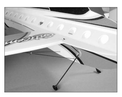
10. Align the skids so they are parallel to the horizontal fuselage and use foam-safe CA to glue the landing gear to the vertical fuselage and wing.
