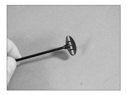
9. Slide the struts through the fuselage and into the slot in the wing. Allow about 3/32-inch (2.5mm) of the strut protruding above the top of the wing.
