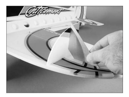
2. Position a 3 ½-inch (80mm) carbon rod between the wing and each of the side force generators. Use foam-safe CA to glue the carbon rods to the wing. Double-check the alignment to make sure the side force generators are square to the wing; then use foam-safe CA to glue the carbon rods to the generators.
