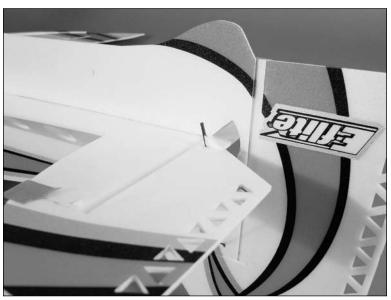
3. Use foam-safe CA to glue the rudder control horn to the rudder. The horn will be on the side opposite the elevator control horn. Again, remove any hinge tape so the horn is glued securely to the rudder.
