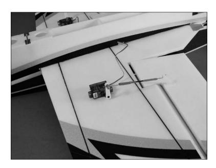
O 14. With the aileron and aileron servo centered, use a 2mm x 4mm machine screw and #0 Phillips screwdriver to secure the pushrod in the connector. Tape the servo lead to the bottom of the wing using hinge tape.
