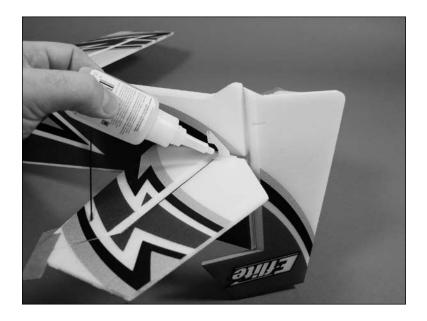
3. Repeat Steps 1 and 2 to install the rudder and aileron control horns.
