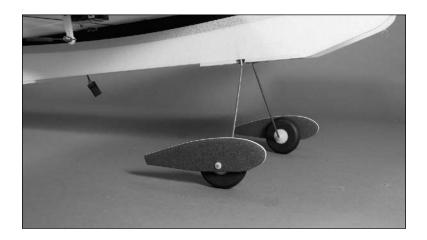
7. Install the landing gear fairings using hot glue. Place a dot of glue at the top and bottom of the fairings to attach them to the landing gear wire.
