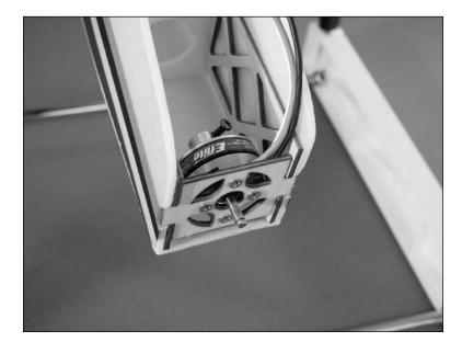
2. Connect the leads from the speed control to the motor.
