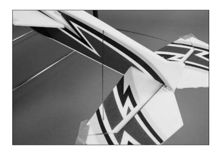
7. Apply hinge tape the the rudder as shown. The tape should not overlap onto the balance tab of the rudder or it will interfere with the operation of the rudder.
