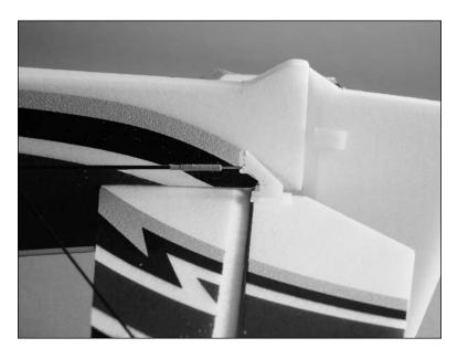
5. Attach the Z-bend on the 10 ½-inch (267mm) carbon pushrod to the middle hole on the rudder control horn.
