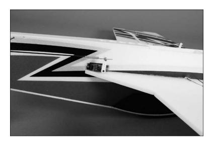
16. With the rudder and rudder servo centered, use a 2mm x 4mm machine screw and #0 Phillips screwdriver to secure the pushrod in the connector.
