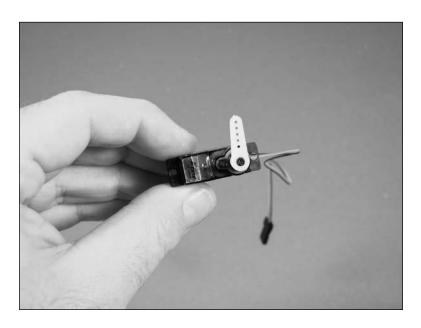
9. Use a pin drill and 1/16-inch (1.5mm) drill bit to enlarge the outer hole in the servo arm.
