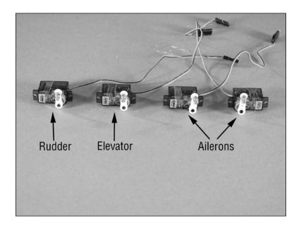
O 13. Slide the end of the aileron pushrod into the micro pushrod connector. Use hot glue to secure the aileron servo to the wing using the servo template on the wing. Another alternative would be to use foam-safe CA to glue the servo down.
