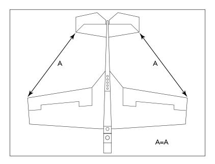
5. Step back and check that the wing and stabilizer are parallel to each other. If not, lightly sand the stabilizer saddle to correct for any alignment issues. Once fully aligned, glue the horizontal stab in place using foam-safe CA.
