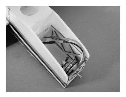
3. Use hook and loop tape to mount the receiver to the side of the horizontal fuselage. Route the antenna wire from your receiver according to the instructions provided with your radio system. Plug the servos into the receiver at this time. Install the speed control in the fuselage using hook and loop tape. Secure the wires so they will not interfere with the operation of the motor during flight.
