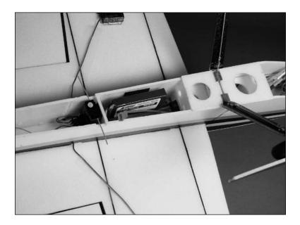
5. Use hinge tape to secure the radio cover to the bottom of the fuselage. Allow the leads for the battery and speed control to exit the cover so they can be manipulated easily without removing the cover.
