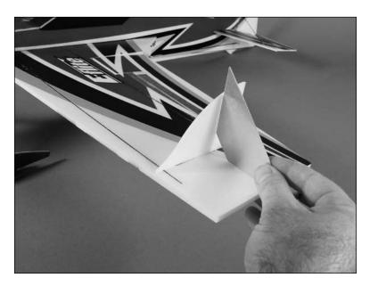
3. Repeat Step 2 to install the bottom side force generator. The bottom will have the tab forward in the slot in the wing.
