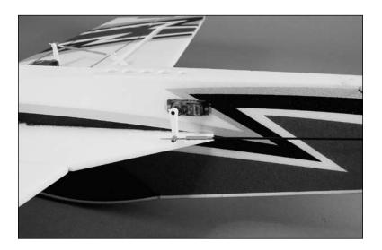
18. With the elevator and elevator servo centered, use a 2mm x 4mm machine screw and #0 Phillips screwdriver to secure the pushrod in the connector. Use threadlock on the screw to prevent it from vibrating loose.
