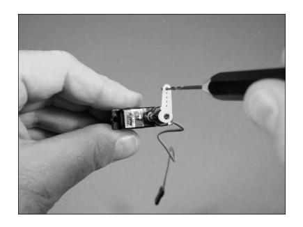
OOO 10. Slide the micro pushrod connector into the outer hole in the servo arm.
