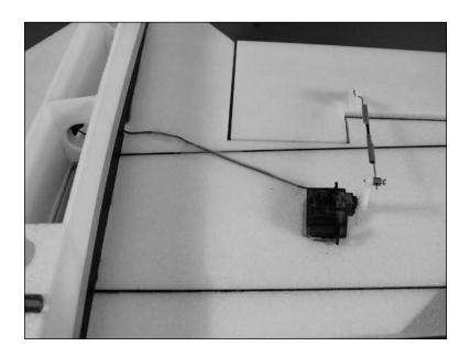
O 15. Secure the rudder servo in the fuselage using hot glue. Slide the rudder pushrod into the micro control connector. Another alternative would be to use foam-safe CA to glue the servo down.
