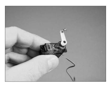
OOO 11. Secure the micro pushrod connector to the servo arm using a micro pushrod connector backplate.
