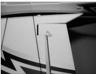
4. Attach the Z-bend on the 10-inch (254mm) carbon pushrod to the middle hole on the elevator control horn.
