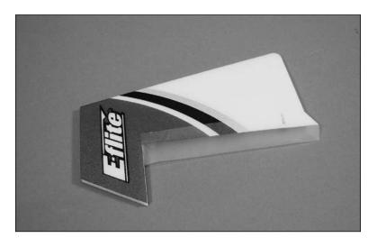
8. Attach the rudder to the fin. Make sure the balance tab on the rudder does not rub against the top of the fin.
