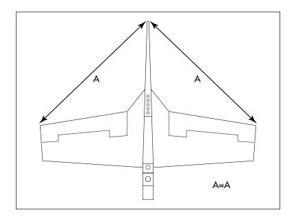
2. Glue the wing to the fuselage using foam-safe CA. Allow the CA to fully cure before proceeding. Ensure the wing is perpendicular to the fuselage during this step.
