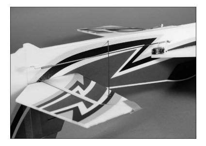
17. Secure the elevator servo in the fuselage using hot glue. Slide the elevator pushrod into the micro control connector. Another alternative would be to use foam-safe CA to glue the servo down.
