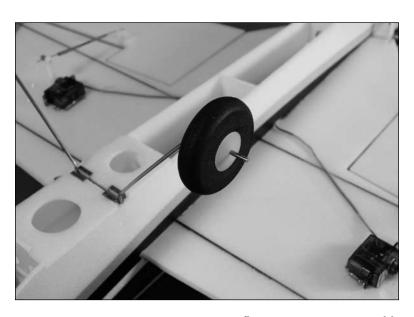
4. Use foam-safe CA to glue the remaining nylon wheel retainer on the landing gear. Use care not to get glue into the wheel and prevent it from rotating.
