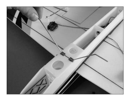
2. Use foam-safe CA to glue the nylon wheel retainer to the landing gear. Make sure to allow the CA to fully cure or you could accidentally glue the wheel to the landing gear.
