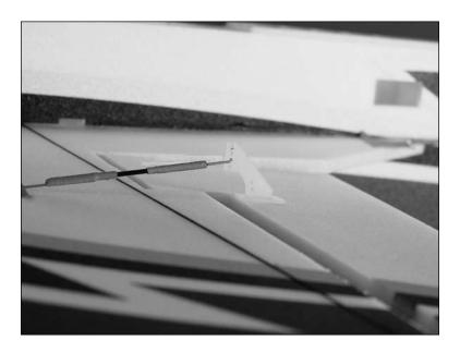
7. Plug the servos into the radio system and make sure they operate and are centered as well. Also center the trims on the transmitter at this time. If you are using a computer radio, start with a clear model program and check that all sub trims are set to 0 and all throws are set to 100%.
