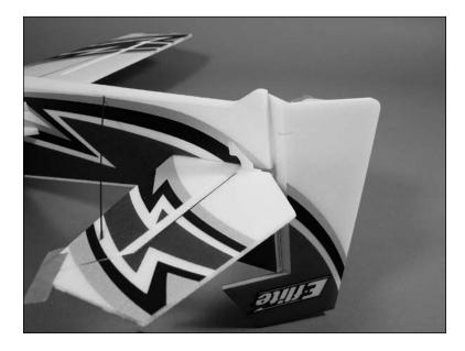
2. Apply a few drops of foam-safe CA onto the backplate to secure it to the horn.
