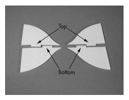
2. Use foam-safe CA to glue the top side force generator into the slot on the top of the wing. Make sure to slide the generator toward the trailing edge of the wing, and that it is square to the top of the wing.
