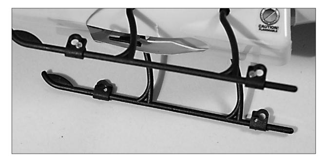
• Locate the four training gear rods and rod mounting base. Note that the rod mounting base has four channels into which the training gear rods will mount. The open side of these channels will face upward toward the bottom of the helicopter when properly installed.
