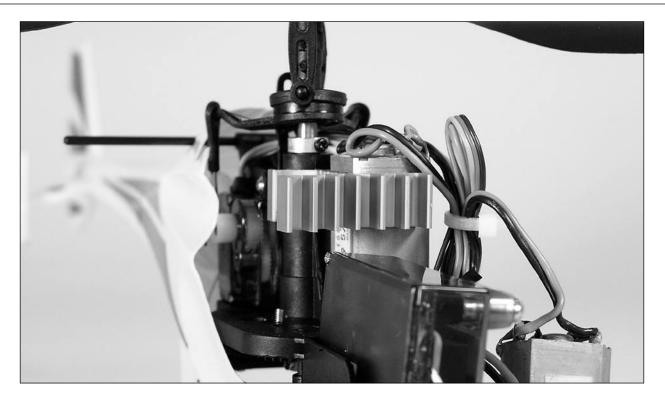
You can now press the right-hand main motor into place in the heat sink and use the motor mounting screws to re-install the motor on the main frame. Again, we recommend that you use Heat Sink Compound (EFLM1913) on any surfaces of the heat sink that make contact with the motor case to further improve the effectiveness of the heat sink.
