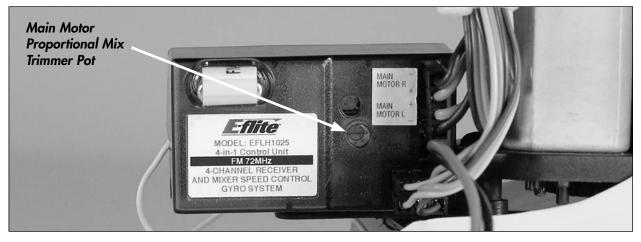
In a stable hover, with the rudder trim centered and no rudder control input, note toward which direction the nose of the helicopter is trying to drift. If the nose of the helicopter is drifting to the left, you will want to increase power to the right-hand motor (spinning the upper main rotor blade). This is accomplished by turning the "proportional" trimmer pot clockwise.
