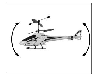
Moving the stick to the left will roll the helicopter to the left, allowing the helicopter to be flown to the left. Moving the stick to the right will roll the helicopter to the right, allowing the helicopter to be flown to the right.
