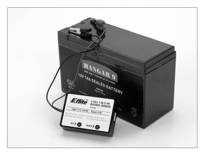
Input power for the charger can also be supplied through the use of an AC to DC adapter/power supply for convenient charging anywhere an AC outlet is available. We recommend the optional E-flite<sup>™</sup> AC to 12V DC, 1.5 Amp Power Supply (EFLC4000). **NEVER attempt to power the charger from an AC outlet without the use of a proper AC to DC adapter/power supply.**
