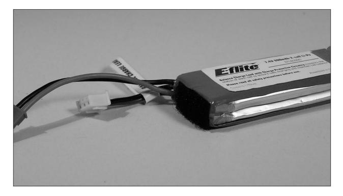
The battery can be installed through the opening in the rear of the body. Be sure to install the end of the battery with the loop material first, with the wire leads oriented to the left side of the model so that they can pass by the stop. Slide the battery into the support frame until the hook and loop material makes contact.
