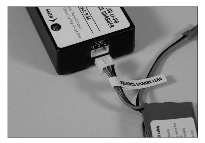
When the battery is properly connected and charging normally, the red and green LED indicators will glow solid. Once the battery has been fully charged, the green LED will go out, leaving just the red LED glowing solid. The battery can now be removed from the charger and installed into the Blade<sup>™</sup> CX for flight.
