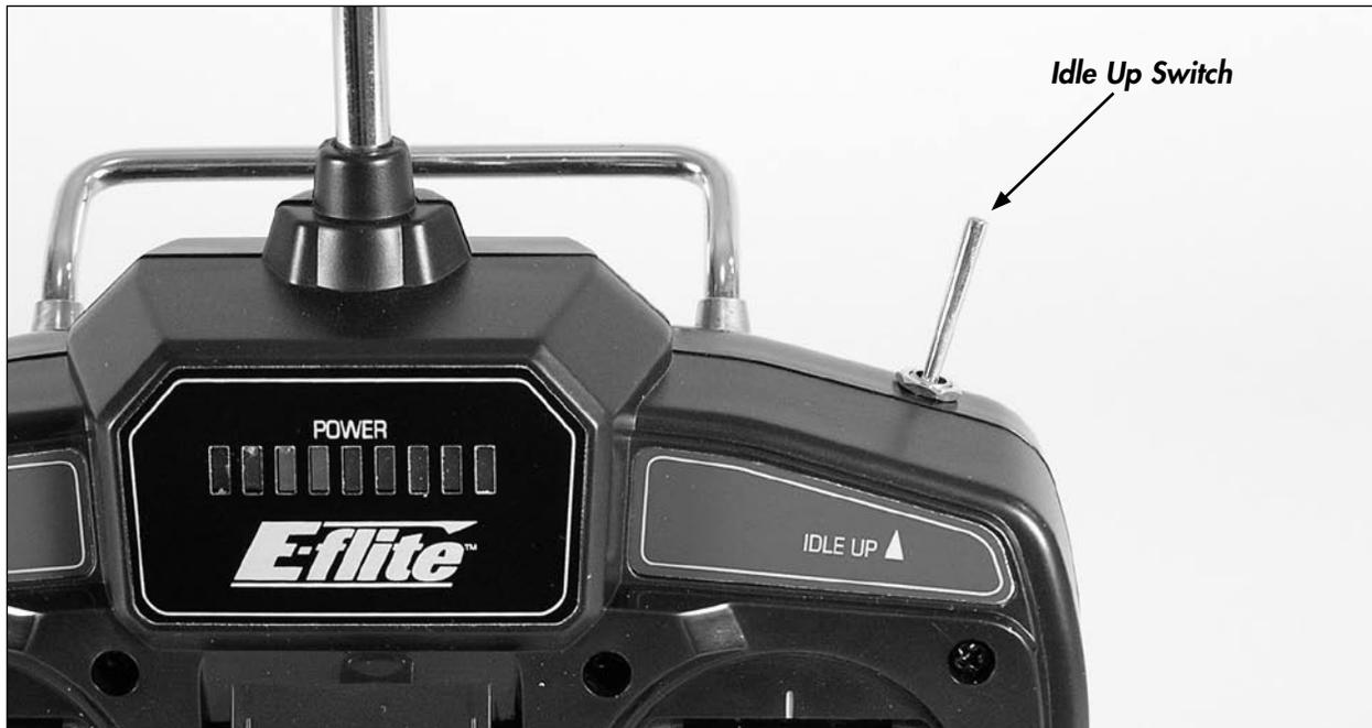
With the switch toggled toward the rear of the transmitter, the Blade CP will be flying in “normal mode.” In this flight mode, the throttle curve is linear from 0% to 100%, with a pitch range of 0 degrees to +10 degrees. (See Page 19 for additional data and graphics relating to the throttle and pitch curves pre-set for your Blade CP.) This is the preferred flight mode for general hovering and gentle forward flight.
