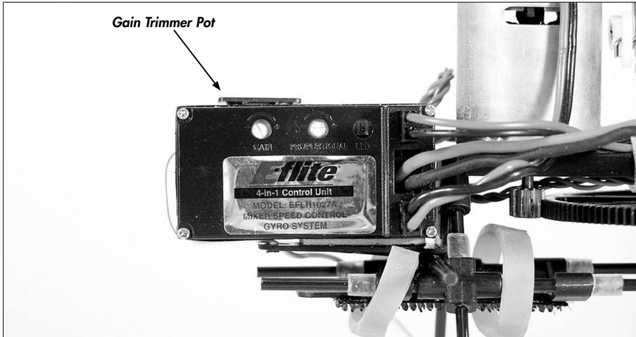
Pilots interested most in hovering-type maneuvers with very little forward flight and aerobatics may choose to have the gain set as high as possible (without making the tail twitch quickly from side to side), keeping the tail of the helicopter very solid during flight. More experienced pilots interested most in fast forward flight and aerobatics may prefer a somewhat lower gyro gain that allows for more control of the tail in flight.
