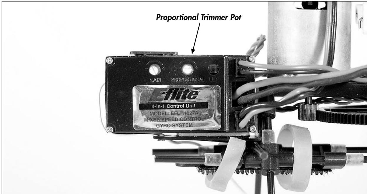
In hover, with the rudder trim centered and no rudder input, note which direction the nose of the helicopter is trying to spin. If the nose of the helicopter is spinning to the left, you will want to increase the amount of tail motor to main motor mixing. By turning the “proportional” trimmer pot clockwise (+), you increase the tail motor/rotor rpm for a given main motor/rotor rpm. This increase in tail motor/rotor rpm will help to push the nose of the helicopter to the right when in hover.
