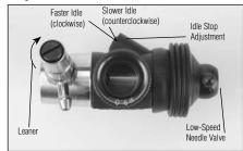
High-Speed Needle: 31/2 turns out (counterclockwise) from closed.
