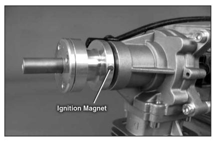
**3.** Next, set the engine at the top of the compression stroke. Note the position of the ignition magnet with engine inverted.
