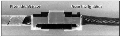
2. Install the silicone wire cover over the pick up lead coming from the engine (cut the excess silicon wire cover) and connect the lead to the pick-up lead from the Electronic Ignition Module. Secure the connection with the included three pin connector securing clip.
