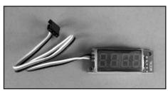
An optional Digital Tachometer is available that can be directly connected to the ignition and display the RPMs of the engine. This unit can be installed on the aircraft or used to spot check the Engine RPMs. Do not install
