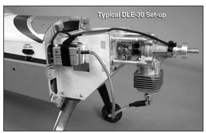
6. Connect the ignition wire from ignition module to the spark plug.
