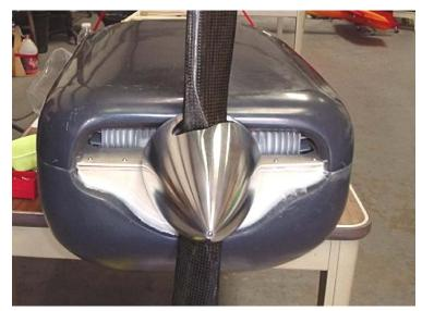
Front cowling inlets guide all incoming air to the upper area of cowl. The same method is used regardless of cowl shape. Air not forced through the cylinders by shrouds and ducting is wasted.
