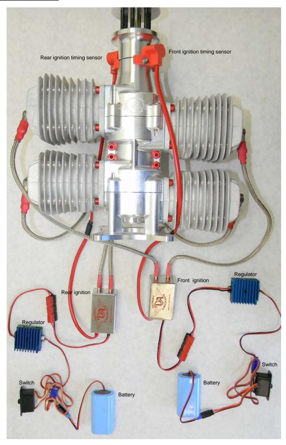
A larger single battery, 1 switch, and 1 regulator, with a "Y" harness to each ignition unit can also be used.
