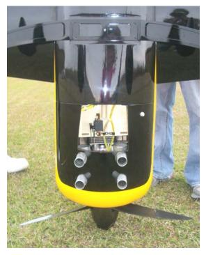
The bottom cowl exit is below and towards the rear, or slightly aft, of the engine. This exit opening should be at least twice the area of the front air inlets. Make sure outside air is not forced into this opening from the bottom of the cowl. A small "lip" extending down from the front edge of the opening can help create a negative pressure area to "pull" hot air out of the exit opening.
