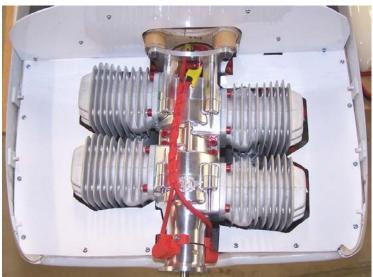
Upper cowling removed showing correct ducting. Notice there is only about a .25"gap around the cylinders and most of the crankcase. All air entering the upper area flows equally down through the fins, then out the bottom cowl exit.
