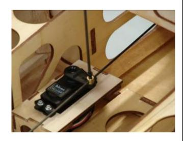
12. Cut off the excess pushrod wire as shown.
