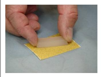
14. Apply thick CA glue to the scuffed side of the silicon rubber piece.
