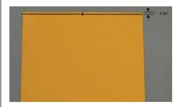
7. Mark a centerline on the bottom of the front former as shown.
