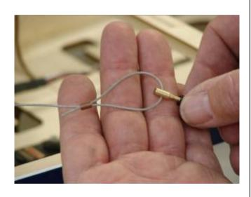
5. Loop the cable back through the brass swage tube as shown.
