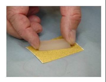
14. Apply thick CA glue to the scuffed side of the silicon rubber piece.
