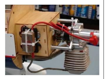
4. Install the ignition battery and regulator if required as desired. A typical installation is shown below. Secure all wiring from excess vibration.
