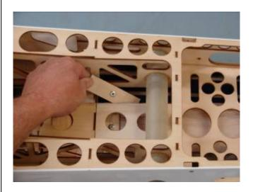
8. Install the canister mounting bolts from inside the canister tunnel and screw into the blind nuts to hold the doublers in place. Do not tighten. Tack glue the edges of the doublers to the top of the canister tunnel with CA glue. Remove the bolts and glue the doublers securely in place. Do not allow CA glue to get into the blind nut threads.
