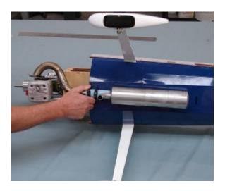
5. Draw a line across the fuse belly on the mark location as shown. This will be the location of the rear former of the canister tunnel.
