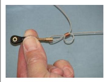
14. Crimp the brass tube with a crimping tool or pliers.
