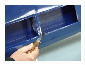
1. Cross braces removed from canister tunnel.
