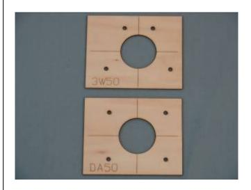
2. Line up the template with the firewall thrust lines and mark the location of the engine mounting holes.
