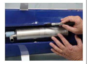
2. Transfer this mark to the top of the canister tunnel. Ensure the mounting holes in the top of the canister tunnel will not interfere with any equipment installed or to be installed inside the fuse.
