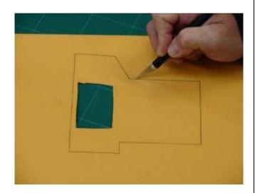
13. With template centered and flush with rear of cowl tape the template to the cowling. Cut the template to clear the air intake on the bottom of the cowl and allow the template to lay flat against the bottom of the cowl.
