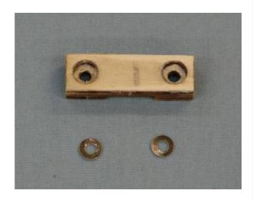
12. Place the flat washers inside the counter sunk holes as shown. Ensure the washer is fully seated inside the counter sunk holes.
