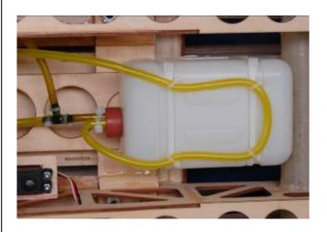
5. Install the fuel filling dot as desired on the side of the fuse. Do not allow the fuel dot to interfere with the leading edge of the wing. Secure the fuel vent line to the front former for proper draining. Drill a fuel line hole in the bottom of the engine box floor to allow fuel pick up line to connect the engine carburetor fuel intake nipple.
