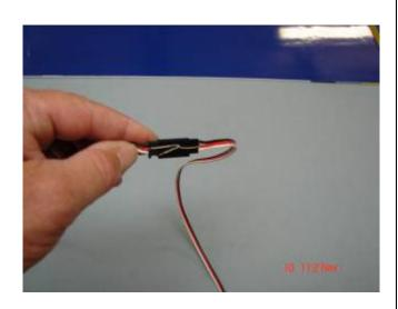
4. Fasten the pull string from the servo hole to the male plug of the servo extension. Secure with tape so that the strings pulls from the front end of the plug. Taper the tape to avoid hang-ups inside the wing.
