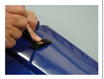
5. Remove servo and use a 1/16 bit to drill servo mounting holes.
