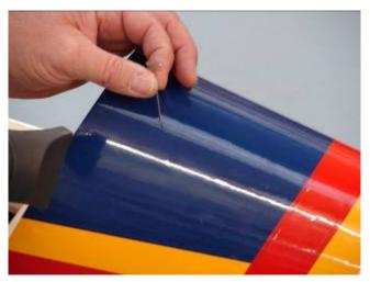
4. Use your heat gun with extreme caution. Take care not to apply too much heat to one area for long periods of time. This may cause the trim colors to over shrink and pull away leaving unsightly gaps on the color lines. The trim stripes are especially vulnerable to over shrinking.
