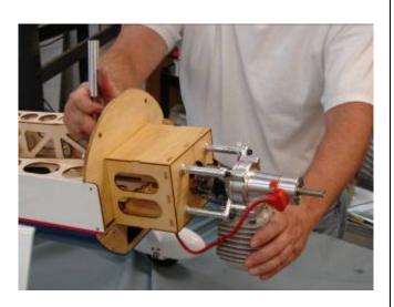
8. Be sure to use flat fender washers on the back side of the firewall to distribute bolt pressure.
