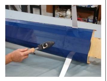
2. Use a hobby knife to remove the covering from the front former to the front of the landing gear cross brace as shown.
