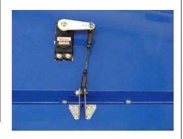
7. Plug the servo wire into the female end of the 36" extension and secure the servo plugs with safety wire, string, tape, or other method. Ensure the plugs will not come apart from vibration or light tension.
