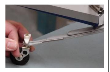
13. Use pliers to twist spring ends closed around the tillers after desired tension and direction adjustments are complete.
