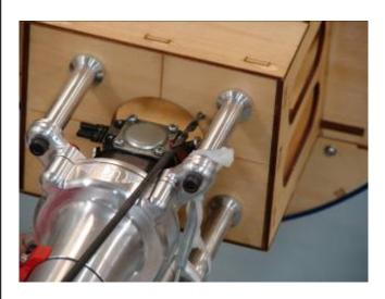
3. Attach the 2-56 ball link to the throttle pushrod and secure to the carburetor throttle arm with a 2-56 bolt and nylon lock nut.
