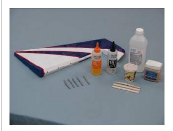
2. Prep all hinges for installation by applying Vaseline petroleum jelly or light oil to the hinge joint. This ensures no epoxy gets into the hinge during assembly.
