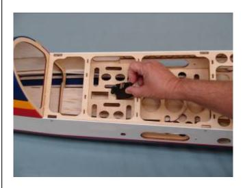
3. Mark and use a 1/16 bit to drill the rudder servo mounting holes.
