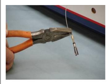
7. If additional crimping is needed a small C-Clamp may be used for additional crimping pressure.
