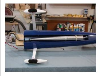
29. Cowl cut out for engine cylinder head with canister and tuned pipe installation. Refer to cowl mounting instructions in the Muffler and Cowl Installation on page 40, steps #1-17.
