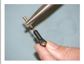
11. Attach ball link to rudder control horn on both sides of the rudder. Thread the rudder cable through a brass swage tube, then the threaded coupler, and back through the brass swage tube on both sides. Pull light tension on the cable through the coupler on both sides as shown. The loop through the coupler should be approximately 1/2" long.
