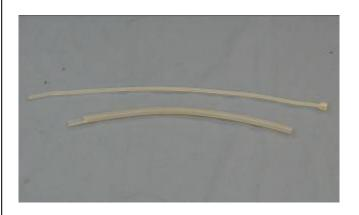
22. Slide the silicon tubing onto the nylon tie as shown to form the pipe strap assembly.
