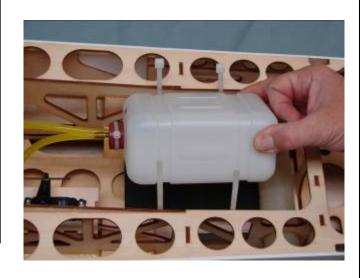
4. Install the fuel tubing as shown with small nylon ties. You will need an after market fuel T and fuel filling dot. Note: We recommend looping the vent line to the rear of the fuel tank as shown to prevent fuel spilling when the model tail is lifted or flying a down line.
