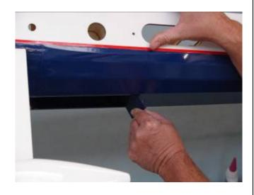
15. Mark the bottom of the fuse line on the former and mark the top of the canister tunnel where the former makes contact.
