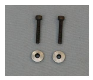
4. Slide the wing tube in the fuse wing tube sleeve. Slide the wings on the wing tube and plug in the aileron servo plugs. Slide the rubber backed washers on the wing mounting bolts and insert bolts through the fuse side and into the wing root blind nuts. Tighten snugly but do not over tighten and crack the fuse or wing root wood.
