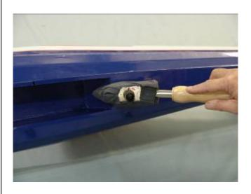
8. Dry fit the header and tuned pipe inside the tunnel and ensure there is clearance on all sides.
