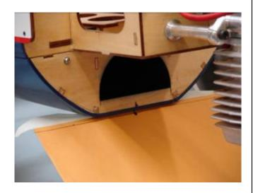
9. Hold the template up to the exhaust stacks and trace the location of the exhaust stacks as shown
