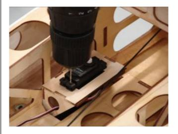
10. Install the servo using servo screws.
