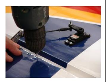
6. Mount the control horn using six wood screws as shown.
