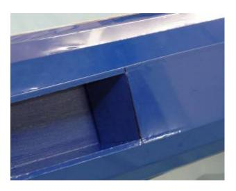
20. Iron the bottom covering to securely seal the covering to the bottom of the rear canister tunnel former.
