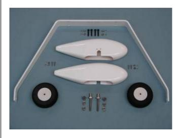
2. Gather the gear strut, 4 mounting bolts, washers, and lock washers, as shown below.
