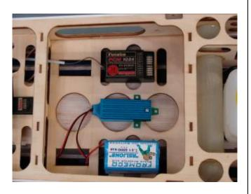
8. Typical installation of RC equipment.
