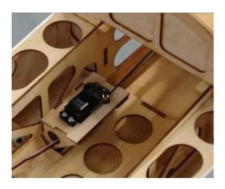
14. We recommend installing the carburetor choke pushrod as shown. Use nylon ties to provide support and holding friction for the choke pushrod. Place silicon fuel tubing over the wire pushrod to prevent damage from vibration and provide holding friction. You can install a choke servo if desired. Use the same mounting steps as the throttle servo.
