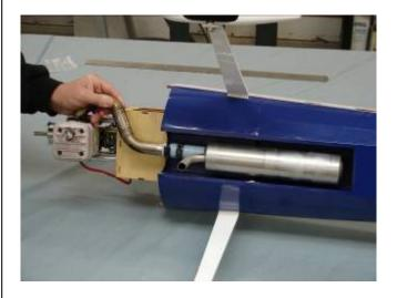
13. Locate the pre-painted balsa canister tunnel rear former as shown below.
