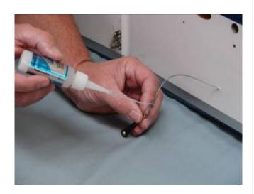
16. Hold the threaded coupler below the cable attach holes to thread into the ball link as shown. Do not hold coupler at the top where the cable hole is located. This may cause burrs on the coupler that can eventually cut the rudder pull cable.
