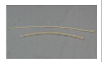
23. Slide the silicon tubing onto the nylon tie as shown to form the canister strap assembly.
