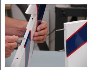
6. Carefully slide the rudder onto each hinge and against the trailing edge of the fin. Wipe away excess epoxy with alcohol wetted wipes.
