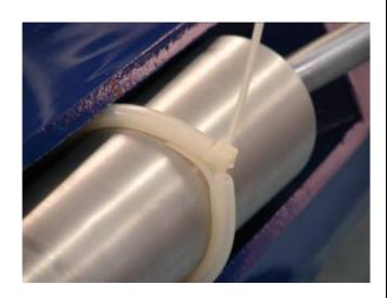
28. Cut off excess nylon tie as shown.
