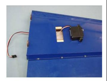
4. Install servo in servo well with the output arm toward the leading edge of the stab and mark locations of servo mounting holes.
