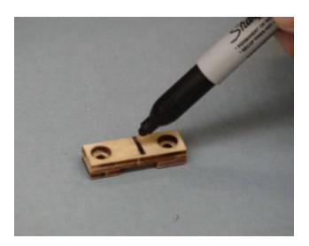
4. Align the centerline of the plywood bracket with the mounting location previously marked on the top of the pipe tunnel. Mark the location of the pipe bracket mounting holes.
