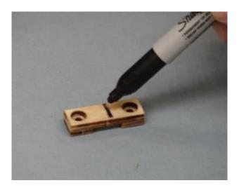
4. Align the centerline of the plywood bracket with the mounting location previously marked on the top of the canister tunnel. Mark the location of the canister bracket mounting holes.
