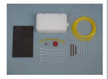
2. Assemble the fuel tank as shown below. Use large diameter tube for pick-up and small diameter tube for the vent. Secure the fuel tubing with nylon ties to the pick-up tube and clunk.
