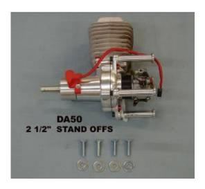
6. Use a drop of blue lock tite on the engine mounting bolts prior to installing.
