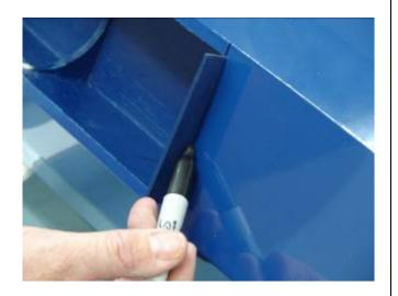
16. Use a hobby knife to cut the former to fit the bottom of the fuse.
