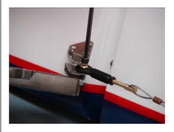
18. Adjust rudder pull-pull cables to desired tension by screwing in or out on the threaded couplers and or ball links. Make all adjustments with the rudder servos still powered up and centered, and the rudder still taped in the neutral position. Ensure the servo does not bind at center or at either end point.
