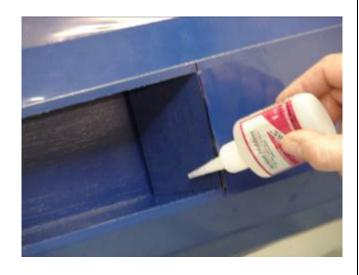
19. Rear canister tunnel former glued in place.
