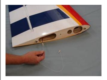
6. Install servo in servo well with the output arm toward the leading edge of the wing and mark locations of servo mounting holes.
