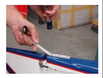
11. Attach the steering springs on both sides of the tail wheel to the rudder tiller and tail wheel tiller. Center the springs between both tillers.
