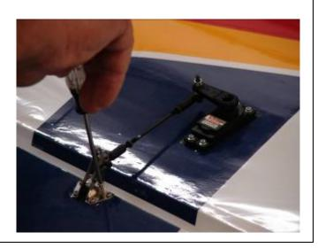
7. Ensure the servo does not bind at either end point at full deflection. A 1" servo arm is recommended for best results. A 1 1/4" servo arm is required for full deflection of the aileron 55° bevel.
