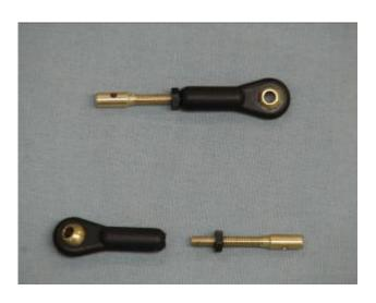
10. Hold the threaded coupler below the cable attach holes to thread into the ball link as shown. Do not hold coupler at the top where the cable hole is located. This may cause burrs on the coupler that can eventually cut the rudder pull cable.
