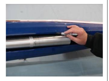
2. Transfer this mark to the top of the tuned pipe tunnel. Ensure the mounting holes in the top of the pipe tunnel will not interfere with any equipment installed or to be installed inside the fuse.
