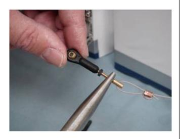
17. Attach ball link to rudder control horn on both sides of the rudder.
