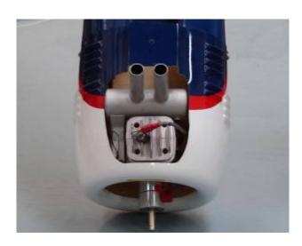
17. Final cowl installation with engine muffler.
