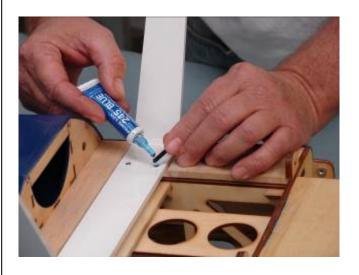
6. Bolt landing gear strut to fuse with 4 bolts and washers. Ensure tapered edge of the gear strut is facing toward the rear.
