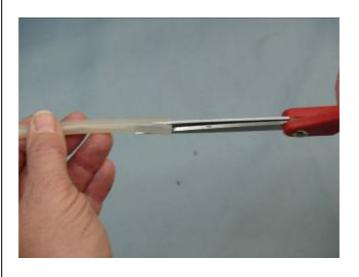
21. After splitting the silicon tubing cut off one side of the split section as shown. This will provide a relief section of the tubing for the nylon tie lock and insulate it from the metal canister surface.
