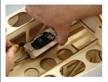
6. Prepare to epoxy the servo mounting tray to the fuse side. Apply epoxy to the back of the servo mounting tray.
