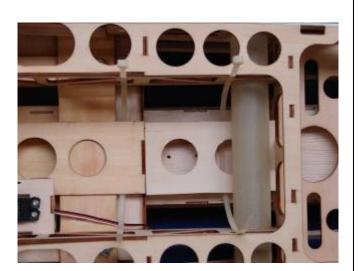
3. Install the fuel tank with foam rubber underneath as shown. Cinch the nylon ties securely to hold the tank against the foam on the fuel tank floor.
