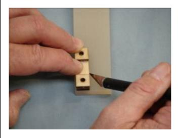
10. Use a hobby knife to cut the flat silicon rubber to match the size of the pipe mounting bracket.
