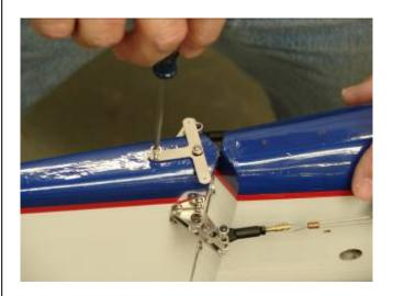
9. Place the tail wheel spring on top of the tail wheel strut. Position the tail wheel and spring on the bottom of the fuse. Place a drop of thick CA on tail wheel strut mounting screws before inserting in the pre-drilled mounting holes on the bottom rear of the fuse.
