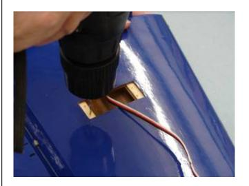
6. Install servo with servo mounting screws.
