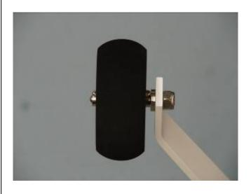
10. Slide the lock washer then the flat washer on the wheel pant mounting bolts. Use blue lock tite on the bolts before final tightening.
