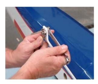
8. Install the inner wheel collar next to the axle bolt. Tighten the inner wheel collar in place. Install the wheel and outer wheel collar. Use blue lock tite on the wheel collar set screw before final tightening.
