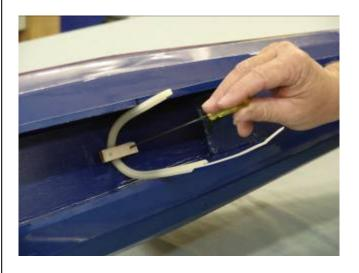
26. Allow the nylon tie lock to extend out of the tunnel 1/1/2" as shown. Tighten the mounting bolts securely.
