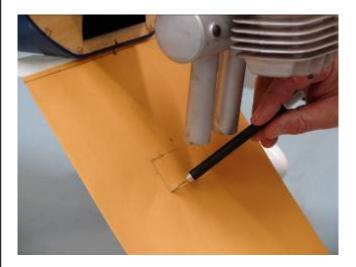
11. Pull up the template to the engine cylinder head and muffler can. Trace around the engine cylinder and muffler can so that they can extend below the template after the tracing is cut out.
