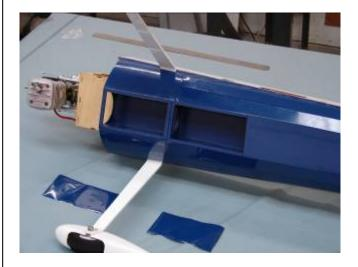
9. Use a razor saw to remove the front former cross brace across the canister tunnel.
