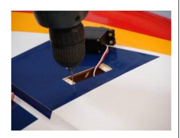
8. Install servo with servo mounting screws.
