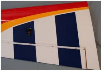
3. Use a ruler against the outboard side of the servo case to project a line to the leading edge of the aileron and mark as shown.
