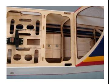
24. Install the pip mounting bolts from the inside the pipe tunnel and screw into the blind nuts to hold the doublers in place. Do not tighten.
