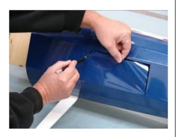
7. Use a hobby knife to remove the covering from the front former to the front of the landing gear cross brace as shown.
