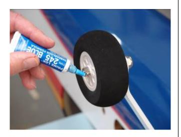
9. Wheel mounted on center of the axle.
