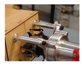
4. The throttle servo is mounted on the side of the fuse that aligns with the engine carburetor throttle arm. Insert the throttle servo into the appropriate throttle servo mounting tray with the output arm forward. Insert the throttle pushrod into the servo arm easy link and dry fit inside the fuse. Align the servo tray so there is no binding on the throttle pushrod.
