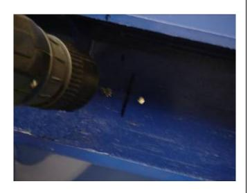
6. Locate the two plywood pipe mounting doublers with pre-installed blind nuts as shown.
