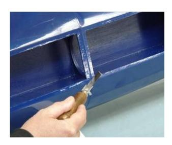
6. Covering and cross braces removed from tuned pipe tunnel.
