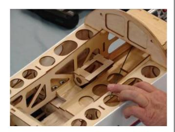
8. Insert the servo into the mounting tray and mark the location of the servo mounting holes.
