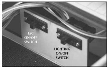
☐ 2. The lighting system has its own dedicated power switch. Turn the power "ON" to illuminate the running lights. If the lights appear to be dim or do not illuminate at all, this is an indication that the batteries need to be replaced.
