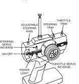
□ 3. Turn the transmitter "ON" using the switch on the front. The red LED light next to the on/off switch should light up. If the LED does not light up, turn the transmitter off and check to make sure that the batteries are installed properly. If you see a
