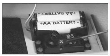
☐ 1. Install two (2) new "AA" batteries into the lighting system battery holder as shown. Be sure to follow the positive (+) and negative (-) pattern molded into the battery holder.
