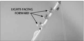
☐ 3. Insert the front mast into the round opening in front of the radio compartment. Gently twist it so that the lights are facing toward the front of the boat.
