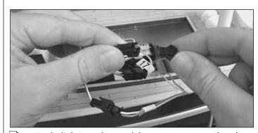
• 6. Each lighting plug and battery connector has been numbered. Plug them into their respective battery connectors. Note: The connectors only fit together one way and the numerical sequence in the photos may not match that of your model.
