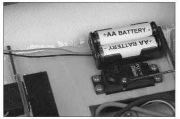
□ 4. Install two (2) new "AA" batteries into the lighting system battery holder as shown. Be sure to follow the positive (+) and negative (–) pattern molded into the battery holder.
