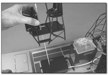
$\ \square$  2. Remove the seat assembly as well as the top of the radio box and lay them to the side.
