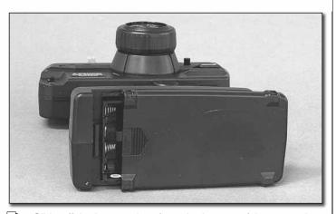
2. Slide off the battery door from the bottom of the transmitter.
