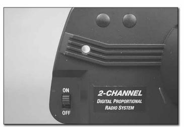
☐ 5. Turn the transmitter "ON" using the switch on the transmitter's left side. The battery level indicator light (LED) should glow green. If the light is flashing the batteries are low and need to be replaced.
