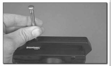
☐ 1. After removing the transmitter and transmitter antenna from the box, line up the antenna to the hole in the top of the transmitter. Slip the antenna in and lightly screw the antenna into the transmitter. Do not over tighten. Give the antenna a light tug to make sure it is properly installed.
