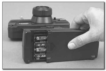
$\square$  4. Reinstall the battery door onto the bottom of the transmitter.
