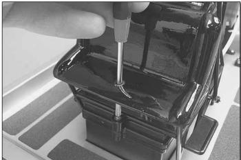
☐ 1. Using a #1 Phillips screwdriver (small), remove the two (2) Phillips head screws from the top of the radio box. One is located under the front seat of the boat and the other behind the back seat.
