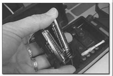
☐ 3. Install 4 "AA" batteries into the battery holder following the diagram in molded in the bottom of the holder.
