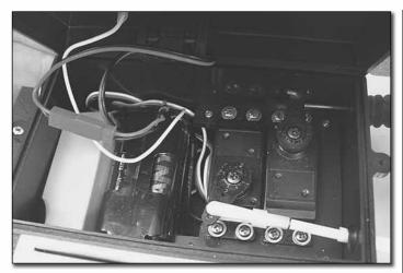
4. Slide the battery box back in the radio box, carefully tucking the wires in the box.
