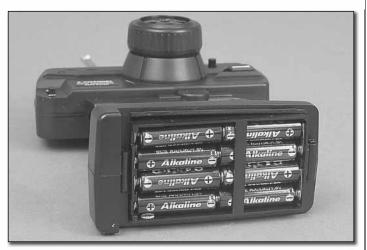
☐ 3. Install 8 "AA" batteries into the transmitter in the configuration molded into the battery floor.
