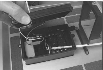
☐ 5. Place the radio box cover as well as the seat assembly in place and reinstall the screws. Be careful to not overtighten.
