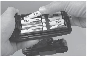
Install eight "AA" batteries into the bottom of the transmitter.
