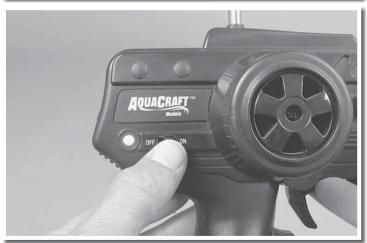
Install the transmitter antenna into the top of the transmitter, turning it clockwise to screw it in place. Then, turn the transmitter on, making sure the power light is glowing.
