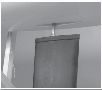
Slip the keel into the hole in the bottom of the hull.
