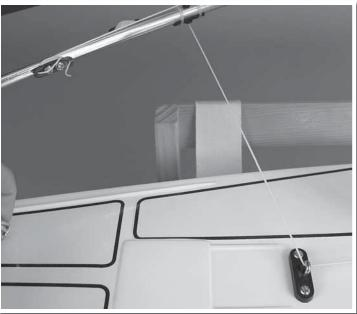
The longer of the winch lines attaches to the jib by slipping the line through the guide on the jib boom and tying off on the forward open cleat.
