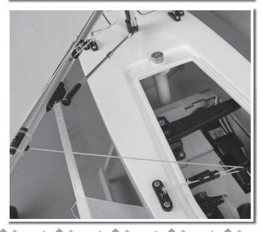
Attach the last of the winch lines to the mainsail by sliding the line through the mast and tying it off on the open cleat on the main boom.
