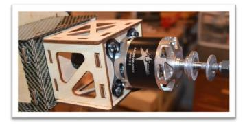
The prop backer plate should be 84-85mm from the motor mounting box. This will provide clearance between the cowl and the motor backer plate.
