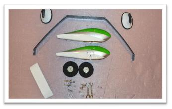
Use the landing gear fasteners (4mm) located on the bottom of the fuselage along with 3 flat washers located in the landing gear package to assemble the landing gear. Add a drop of removable thread locker to the screws during assembly.
