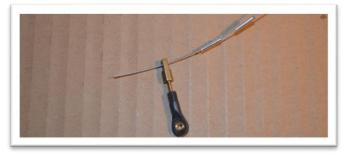
Loop around the cable eye and go back through the first crush sleeve.
