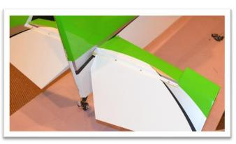
Attach a 24" servo extension onto the elevator servo lead and use shrink wrap or a safety clip to secure the connection.
