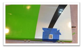
Use sand paper to roughen up the control horns so the epoxy will adhere better. Assembly the control horns with a ball link and brass cable eye. Thread the cable eyes about half way into the ball link.
