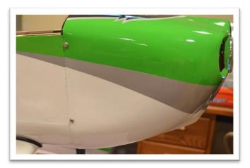
Remove the cowl and apply thin CA glue to the mounting tabs and screw holes. (Allow plenty of time for the CA glue to dry before reinstalling the cowl.)
