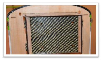
Use 4mm bolt and washer on the front and a nylon lock nut and washer on the back to secure the motor box to the fire wall. Apply removable thread locker to the bolts during assembly.
