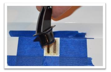
Wipe away excess epoxy using a paper towel soaked with denatured alcohol. Use an upward rolling motion as you wipe the excess epoxy to lift it from the surface. This helps reduce smearing the epoxy.
