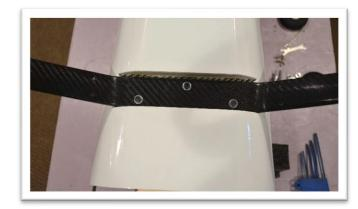
Place the wood filler block over the landing gear. We suggest using a piece of white covering or clear packing tape to hold the filler block in position.
