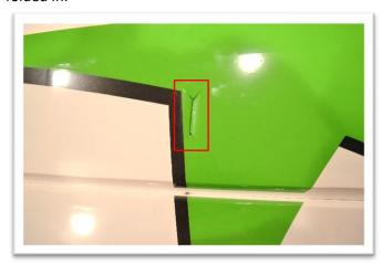
Gently snap off the servo wire installation string and temporarily secure it out of the way. Do not pull it out of the wing.
