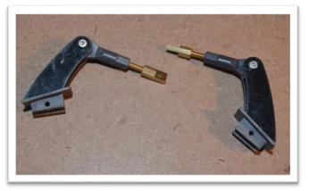
Tests fit the control horns to the slots and align with the hinge line. The control horns should be symmetrical about the hinge line.
