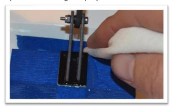
Check the alignment along the hinge line as you did when you test fit the control horn. Reposition as needed. Allow the epoxy to partially cure. Peel away the masking tape after the epoxy is securely holding the control horn in place and still soft enough to easily remove the tape. Set aside and let the epoxy fully cure. (Repeat on second elevator half if you will be using 2 elevator servos.)
