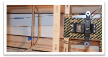
Center the rudder and position it aligned to the vertical stabilizer. Tape the rudder to the vertical stabilizer to hold it centered.
