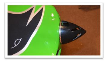
The prop backer plate will be 160-161mm from the fuselage firewall.
