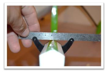
Use 30 minute epoxy to glue the control horns in place. Check the alignment, peal the masking tape away and set aside for the epoxy to cure.
