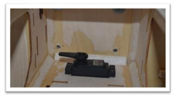
The servo could also be mounted to the side for the fuselage by adding a couple pieces of hard balsa or spruce.
