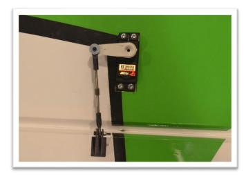
Adjust the position of the aileron to the wing by turning the turnbuckle. You do not need to disconnect it from the servo or control horn.
