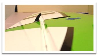
Allow the epoxy to partially cure. Peel away the masking tape after the epoxy is securely holding the control horn in place and still soft enough to easily remove the tape. Set the wing aside and let the epoxy fully cure.
