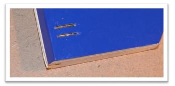
Test fit the control horn halves in the slot individually, then as an assembly. The fit should be snug. Check the alignment of the control horn to the hinge center line as you did with the wing. The linkage hole in the control horn should be aligned with the hinge centerline.
