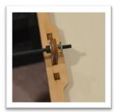
Secure the canopy to the fuselage with the 3mm thumb screws and flat washers.
