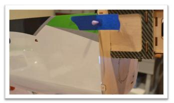
Peal back the tape to uncover the mounting tabs and install the cowl but leave the tape on the fuselage. Tape the cowl into position centering it to the motor using your spinner's back plate as a guide and aligning it to the top edge of the firewall.
