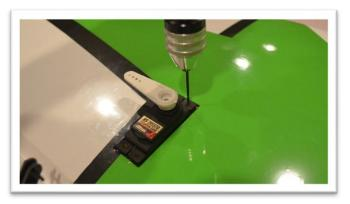
Thread 2 rod ends on to a turnbuckle connecting rod engaging half the threads into the rod end. Notice that one end of the rod has a right hand thread and the other end has a left hand thread. This allows you to adjust the connecting rod without removing it.
