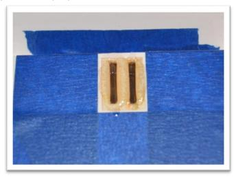
Apply epoxy to the control horn assembly and insert it into the aileron slots.
