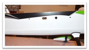
Carefully locate the horizontal stabilizer pocket. Use a trim iron to seal the covering around the edges of the pocket before trimming. Use a new hobby knife blade to cut though the covering.
