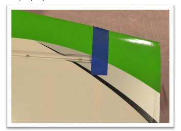
Carefully remove "masking" tape before the epoxy fully sets. But do not remove the tape at the stabilizer and elevator counter balance until epoxy is fully cured.
