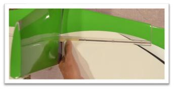
Apply petroleum jelly (Vaseline) to the center hinge pin portion of each hinge. This will help prevent glue from getting into the hinge when gluing then into the elevator. Avoid getting petroleum jelly on the barbed portion of the pin. If you do clean it off with alcohol.
