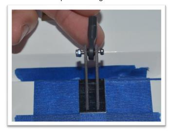
Remove the control horn leaving the tape in position. Using a new hobby knife blade and lightly cut through the covering but not into the balsa sheeting.
