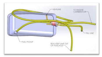
Position the fuel tank in front of the wing tube. Placing a piece of foam under the tank will prevent fuel foaming from vibration. Secure the tank using the hook and loop straps running through the slots on the plywood tray. We recommend using at least a 1" strap if you intend to do high G, 3D maneuvers.
