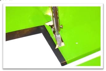
Carefully locate the aileron control horn slots. Use a covering sealing iron to bond the covering in the area the control horn will sit. Trim the covering away to expose the slots. Be careful you don't cut through to the top side covering.
