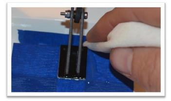
Check the alignment along the hinge line as you did when you test fit the control horn. Reposition as needed.
