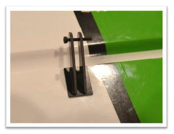
Check the alignment of the control horn to the hinge center line. The linkage hole in the control horn should be aligned with the hinge centerline.
