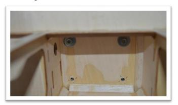
The distance between the prop backer plate and the firewall should be 160-161mm. This will provide space between the spinner and the cowl.
