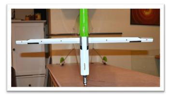
Push the horizontal stabilizer all the way forward in the pocket. Position the stabilizer parallel to the main wing tube. Adjust the stabilizer until the measurements to the wing tube are equal on both sides. Continue checking the stabilizer to ensure it is still centered as described above. Extra time spent here will go a long way to improve the flight characteristics of your airplane.
