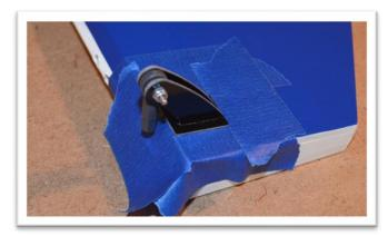
Remove the control horn leaving the tape in position. Using a new hobby knife blade lightly cut through the covering but not into the balsa sheeting. Cut inside the tape edge about 1/16".
