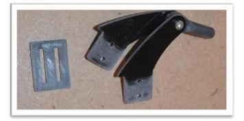
Apply epoxy to the slots in the elevator. Use a pin to help push some epoxy into the slots.
