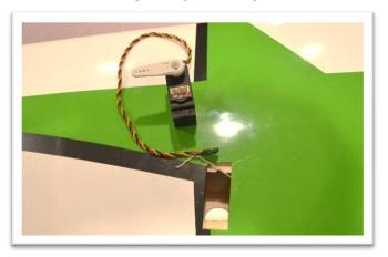
Pre-drill for the servo mounting screws using a 1/16" drill bit. Install the servo with the wood screws that came with your servos. Remove the screws and servo. Apply a drop of thin CA glue into each mounting screw hole. This will harden the wood around the screws and provide a more secure installation. (Allow the CA glue to dry before reinstalling the servo.)
