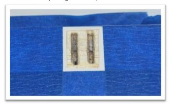
Use sand paper to roughen the lower portion of the control horns on both sides. Roughen one side of the base plate. This will help the epoxy bond to the control horn parts.
