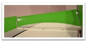
A small round file can be used to give the hinges some clearance. Cleaning out the holes will also help you close up any gap. Turn a 1/8" drill into the holes by hand.
