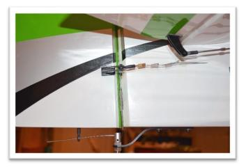
Remove the tape from the rudder/vertical stabilizer. Adjust the length of the cable by turning the brass cable eyes to center the rudder and achieve the desired cable tension.
