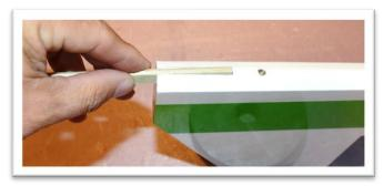
Insert hinge pins into the elevator halves and the horizontal stabilizer. Check the fit and gap at the hinge line. You may need to adjust the hinge holes to minimize the gap.
