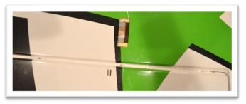
Use the control horns from the "Wings" part bag. Test fit the control horn in the slot. Trim or file the slot as needed to achieve a snug fit. Make sure the shoulder of the control horn is fully seated down against the control surface.
