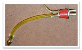
Insert the assembly into the fuel tank and check that the clunk if free to move around. Rotate the tank side to side and upside down to ensure the clunk does not get stuck. If cluck does not move freely in all positions trim a little off the fuel line and try it again. When you have established the correct length of the fuel line you can tighten the stopper screw.
