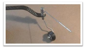
Use the landing gear fasteners (4-40) locate on the bottom of the fuselage along with 2 flat washers located in the landing gear package to mount the carbon fiber landing gear. Add a drop to removable thread locker to screws during assembly.
