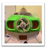
Drill a 1/16" hole in the cowl through the locating holes you created in the tape.
