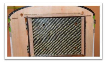
Drill the mounting holes for your engine then temporarily mount it engine standoffs. (A DLE35RA is shown on the 73" AJ Laser which is very similar..)
