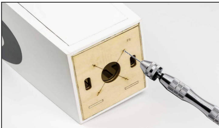
参考马达座的螺丝孔位，在机身头部钻出四个引导孔。 Refer to the screw's hole position of motor mounting board, drill 4pcs holes on the head of fuselage.
